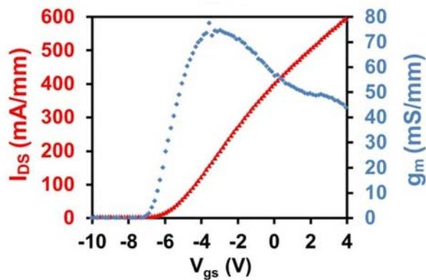
Fig. 4: Transfer characteristics of the AlGaIn/GaN MOS-HEMT
