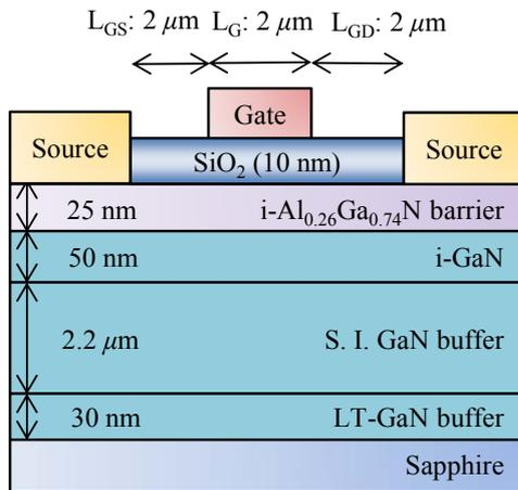
Fig. 2: Cross-sectional view of the fabricated AlGaIn/GaN MOS-HEMT
