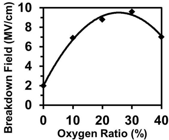
Fig. 1: Breakdown field of the sputtered-SiO<sub>2</sub> films on n<sup>+</sup> GaN as a function of oxygen ratio
