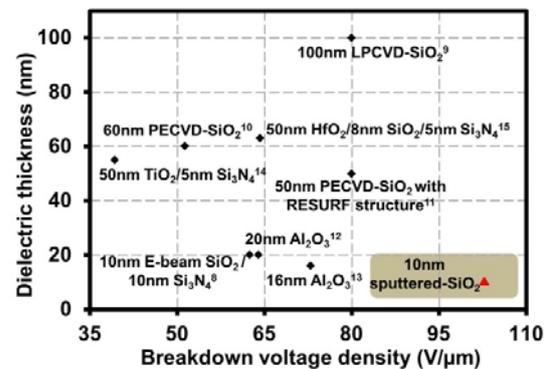
Fig. 5: Comparison of breakdown voltage density of MOS-HEMTs achieved by different groups
