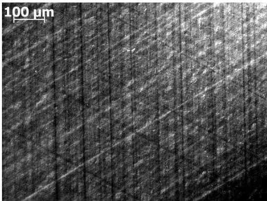
Figure 1: Nomarski microscope image of plastically deformed GaN on Silicon.
