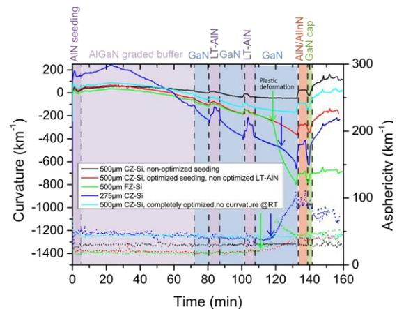
Figure 2: Curvature measurements of an AlInN/GaN HEMT structure grown on Si(111) substrates. The parameter variation (type of substrate, seeding, LT-AlN) is given in the insert (solid). In addition, the asphericity of the wafer is measured simultaneously (dotted).
