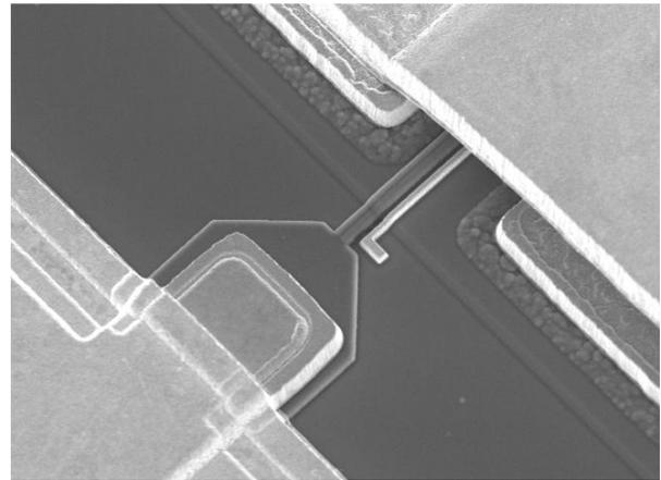
Fig. 3 0.2µm dual field plate GaN device.
