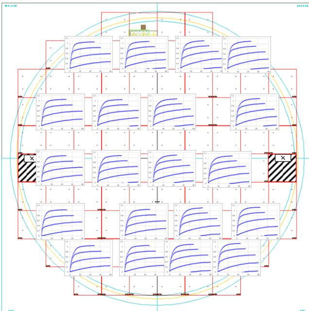
Fig. 4 Mapping of 0.2µm GaN HEMT pulsed I-V
