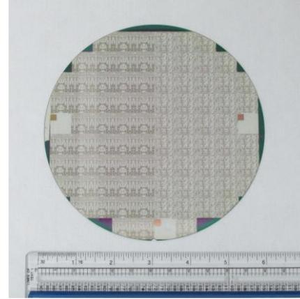
Fig. 1 A fabricated 6" GaN HEMT MMIC wafer.
