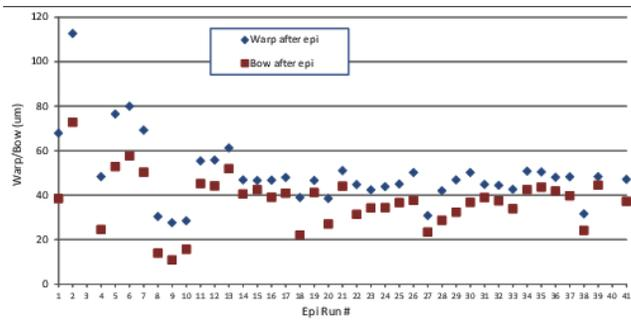
Fig. 2 Improved warp/bow (~40µm) from 6" GaN epi wafers.
