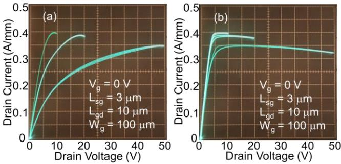
Fig. 3 Drain I-V characteristics measured at  $V_g = 0$  V while varying drain voltage swing from 10 to 50 V for devices (a) without and (b) with  $O_2$  plasma treatment.
