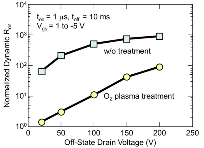
Fig. 5 Normalized dynamic  $R_{on}$  as a function of off-state drain voltage for devices with and without  $O_2$  plasma treatment. On-state duration time is 1  $\mu$ s.
