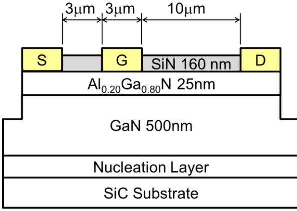
Fig. 1 Cross sectional view of fabricated AlGaIn/GaN HEMT.
