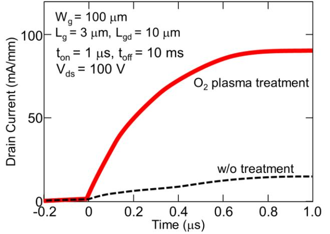
Fig. 4 Transient drain current waveform for devices with and without  $O_2$  plasma treatment. Off-state drain bias voltage is 100 V.
