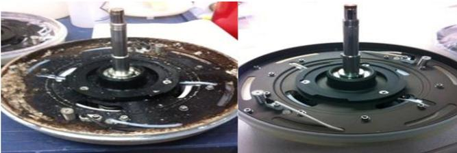
Figure 3. Plating rotor before and after “in house” repair.
