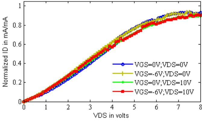
Fig. 3. Normalized Pulse IV data for the HEMT devices on Sapphire with 10% duty cycle probed from various bias points.
