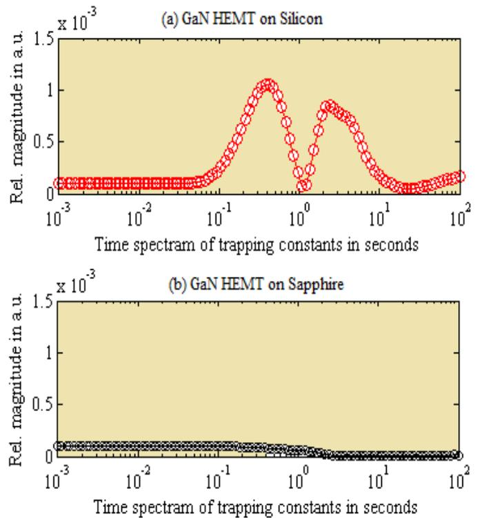
Fig. 8. Emission time constant spectra analyzed from transient after a deep OFF-state pulse.
