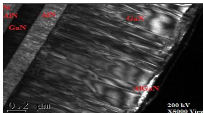
Fig. 2. Bright Field cross sectional imaging of the device layers grown on Silicon showing a dislocation density in the order of  $10^{10}/\text{cm}^2$  (TEM image for Sapphire not shown)
