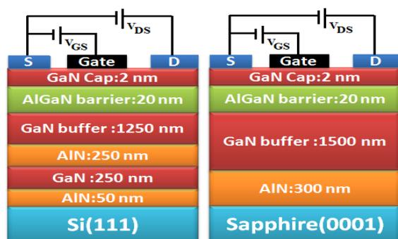
Fig. 1. Representative epitaxial structures of the HEMTs grown on Silicon and Sapphire.
