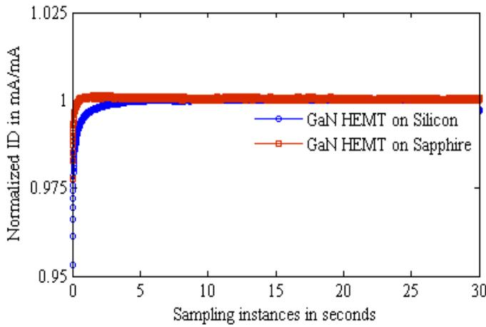
Fig. 5. Normalized current transient for HEMT devices sampled after a high on-state pulse.
