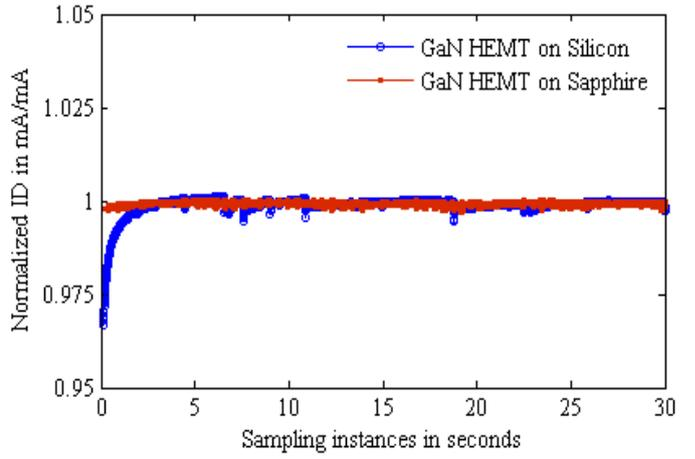
Fig. 6. Normalized current transient for HEMT devices sampled after a high on-state pulse.
