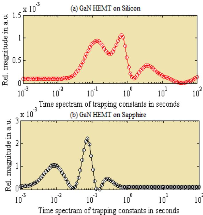
Fig. 7. Emission time constant spectra analyzed from transient after a high ON-state pulse.
