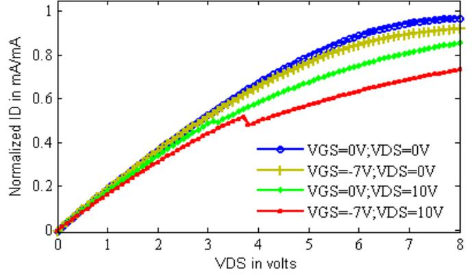
Fig. 4. Normalized Pulse IV data for the HEMT devices on Silicon with 10% duty cycle probed from various bias points.
