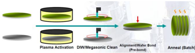
Figure 1: Fusion wafer bonding process flow
