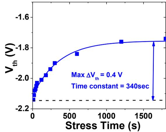
Figure 2. The threshold voltage and the fitted curve of the SBD with different off-state stress time.
