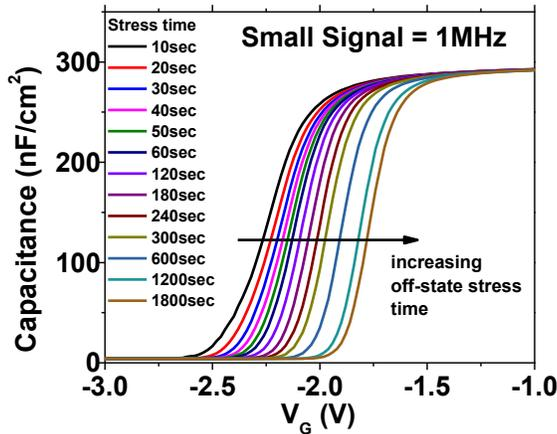
Figure 1. The measured C-V characteristics of the SBD after different stress time.
