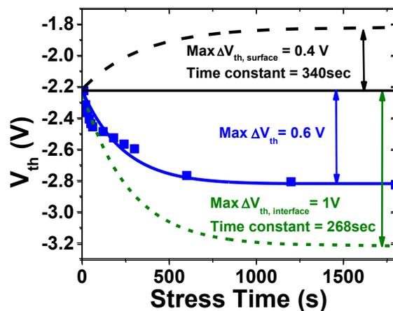
Figure 6. The threshold voltage and fitted curves of the MISC after different stress time.
