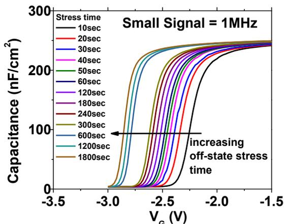
Figure 4. The measured C-V characteristics of the MISC after different stress time.
