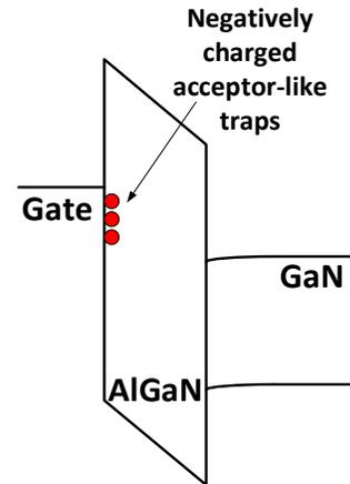
Figure 3 Band diagram of AlGaIn/GaN heterostructure showing the formation of negatively charged acceptor-like traps at off-state stress ( $V_{GS} = -5V$ ).
