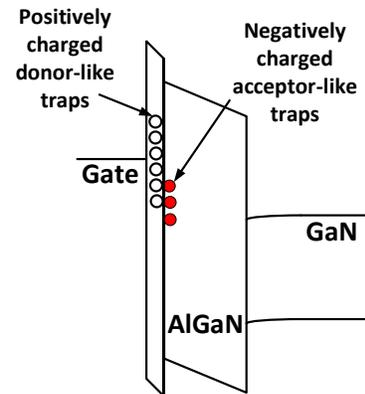
Figure 5 Band diagram of  $\text{Al}_2\text{O}_3/\text{AlGaIn}/\text{GaN}$  heterostructure showing the formation of negatively charged acceptor-like surface trap and positively charged donor-like traps at off-state stress ( $V_G = -5 \text{ V}$ ).
