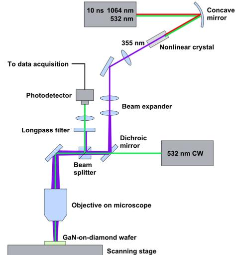
FIG. 1. Schematic of the transient thermoreflectance measurement setup.
