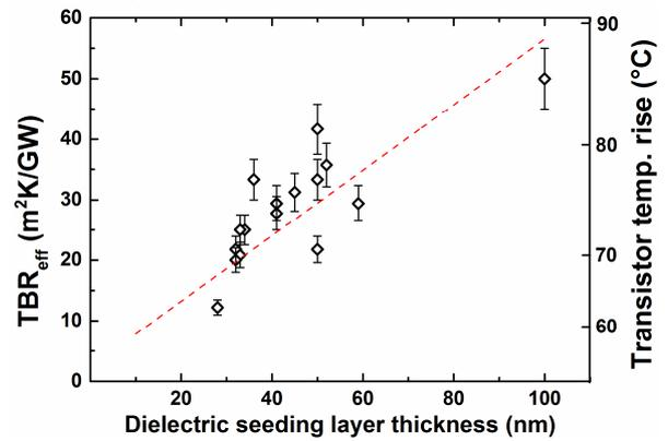
FIG. 4.  $TBR_{eff}$  of the GaN/diamond interface as a function of the dielectric seeding layer thickness. The corresponding transistor peak channel temperature rise is indicated on the right vertical axis. A straight line is shown for visual guidance.
