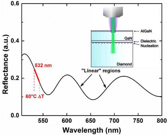
FIG. 2. Measured reflectance spectrum of a GaN-on-diamond wafer as a result of the partially coherent internal reflections of the probe laser, as illustrated in the inset. The 532 nm wavelength is within the regions where a linear approximation between reflectance change and surface temperature rise is valid.
