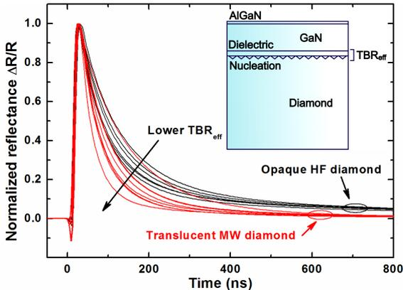
FIG. 3. Normalized transient reflectance of GaN-on-diamond wafers with different thicknesses of the dielectric seeding layer. Two diamond growth methods were used: Hot filament (HF) CVD and microwave (MW) plasma CVD. Inset shows a schematic of the sample layer structure.
