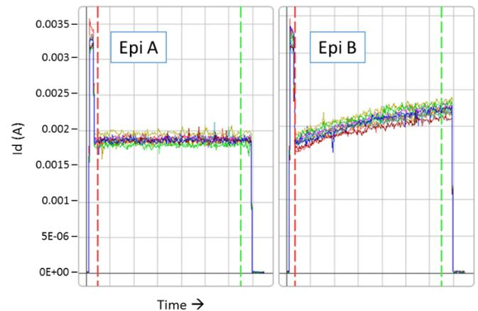
Figure 2: Transient response of device from two epi wafers under DEVM conditions
