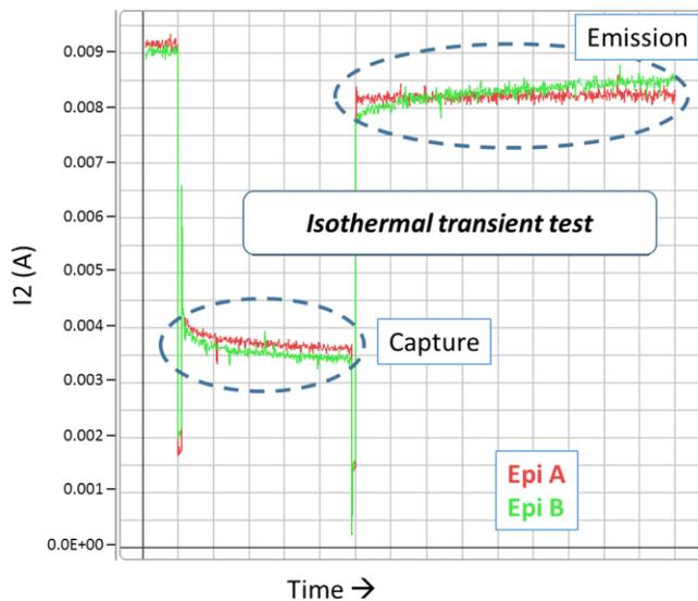
**Figure 4:** Transient response for test 2, isothermal transient test on two epi types
