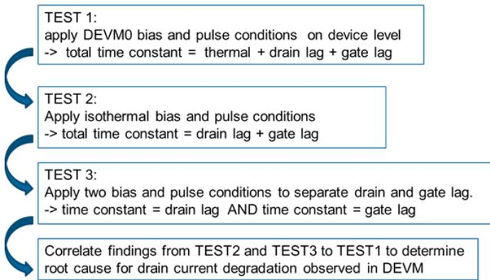
**Figure 3:** Test flow for transient characterization
