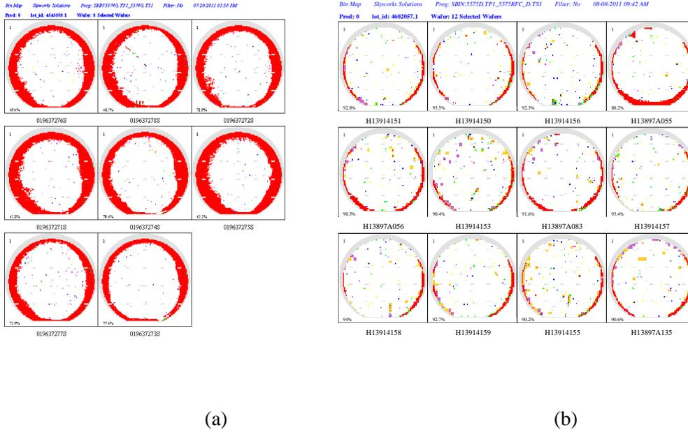
Fig. 2. Probe test data shows minimized edge yield loss due to oxygen contamination. (a) Old process; (b) Modified process.
