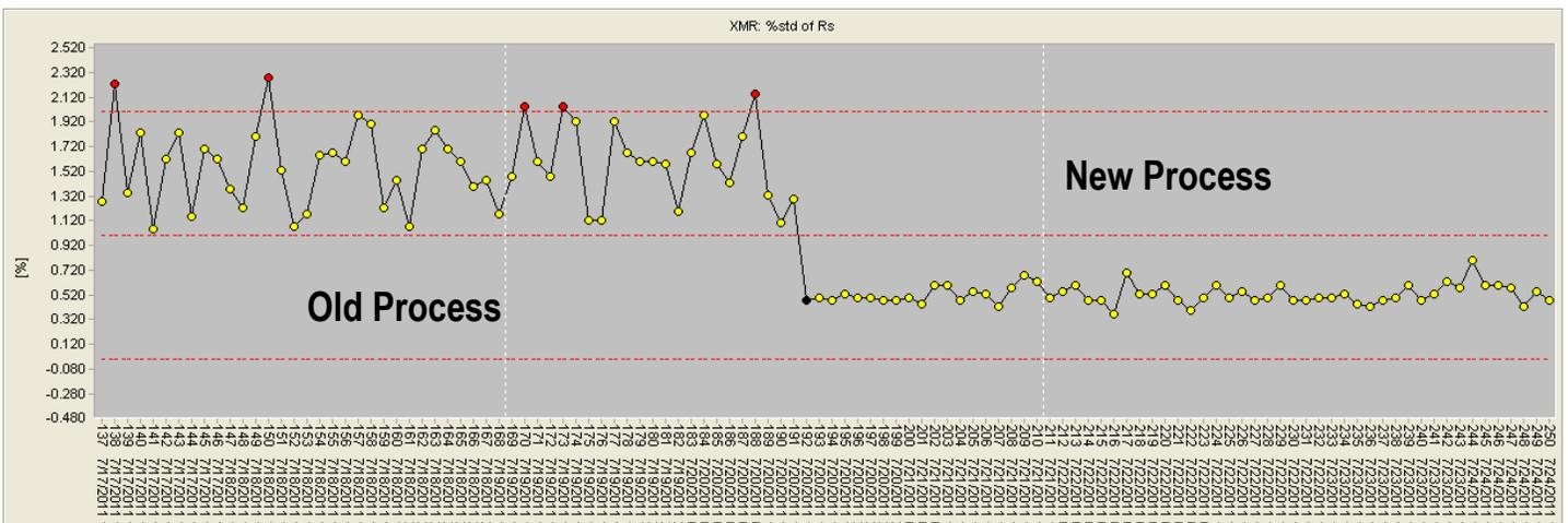
Fig. 3. Standard deviation of sheet resistance SPC chart shows improvement after the implementation of new growth process.
