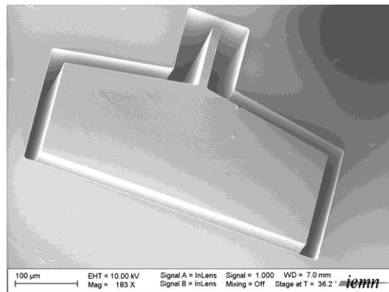
Fig. 1: Schematic cross section of the AlN/GaN/AlGaN DHFET with the local substrate removal and SEM picture of the back-side ring around the drain after the silicon etching
