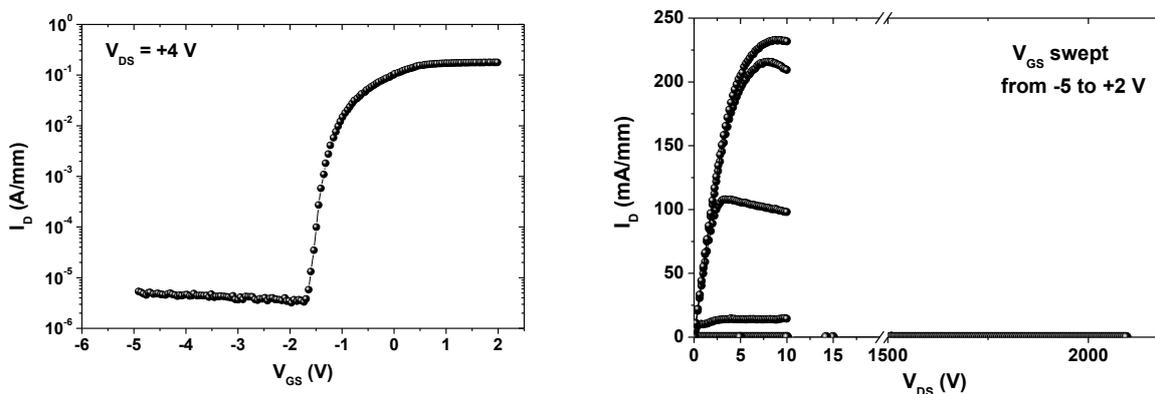
Fig. 2: Transfer characteristic at  $V_{DS} = 4V$  (left) and  $I_D$ - $V_{DS}$  characteristics (right) of a  $1.5 \times 50 \mu\text{m}$  AlN/GaN-on-Si DHFET with  $L_{GD} = 30 \mu\text{m}$  after local substrate removal.
