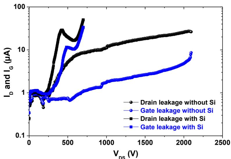
Fig. 3: Off-state characteristics of a  $1.5 \times 50 \mu\text{m}$  AlN/GaN DHFET with  $L_{GD} = 30 \mu\text{m}$  before and after local substrate removal at  $V_{GS} = -5V$ .
