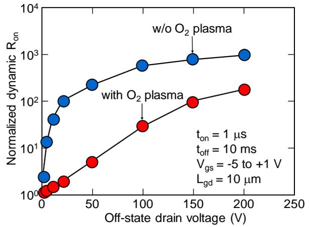
Fig. 2 Normalized dynamic  $R_{on}$  as a function of off-state drain voltage for devices with and without  $O_2$  plasma treatment. On-state duration time is 1  $\mu s$ .
