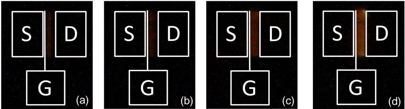
Fig. 3 Luminescence evolution of  $O_2$  plasma-treated device ( $L_{gd} = 25 \mu m$ ) with increasing  $V_{ds}$ : (a)  $V_{ds} = 800 V$ , (b)  $V_{ds} = 1200 V$ , (c)  $V_{ds} = 1500 V$ , (d)  $V_{ds} = 1800 V$ .
