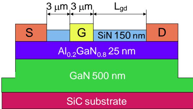
Fig. 1 Cross section of fabricated AlGaIn/GaN HEMTs.
