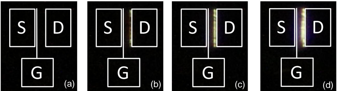
Fig. 4 Luminescence evolution of device ( $L_{gd} = 25 \mu m$ ) without  $O_2$  plasma treatment with increasing  $V_{ds}$ : (a)  $V_{ds} = 800 V$ , (b)  $V_{ds} = 1000 V$ , (c)  $V_{ds} = 1200 V$ , (d)  $V_{ds} = 1400 V$ .
