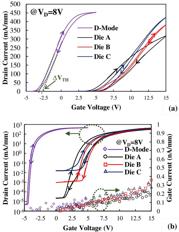
**Fig. 2 (a)** Bi-directional transfer characteristic of Dies A-C with benchmarking D-mode device in linear scale. The sweep was done in 20s and threshold voltage hysteresis ( $\Delta V_{TH}$ ) is demonstrated. **(b)** Bi-directional transfer characteristic in logarithmic scale and  $I_G$ - $V_G$  characteristics of Dies A-C and D-mode device. Low gate leakage current has ensured the preservation of insulation quality of the gate dielectric with fluorine treatments.
