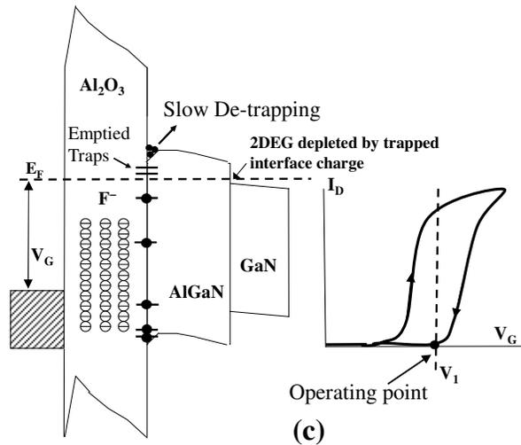
**Fig. 5** Schematic energy band diagram of  $\text{Al}_2\text{O}_3/\text{AlGaN}/\text{GaN}$  interface at (a)  $V_G=0\text{V}$  (leakage current induced by hole trapping in shallow  $D_{it}$  and hopping across the gate region into the channel) (b)  $V_G=V_1$  in positive sweep (trapping of  $Q_{it}$  from 2DEG) and (c)  $V_G=V_1$  in negative sweep (2DEG depletion from  $Q_{it}$  resulted in positive  $V_{TH}$  shift)
