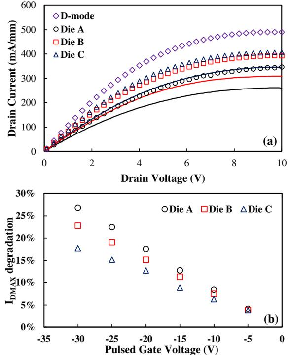
**Fig. 3 (a)**  $I_D$ - $V_D$  characteristic of Dies A-C with benchmarking normally-on device at gate drive voltage in excess of  $V_{TH}$  ( $V_{GT}$ ) of 10V in DC state (datapoints). Pulsed  $I_D$ - $V_D$  (solid line) measured
