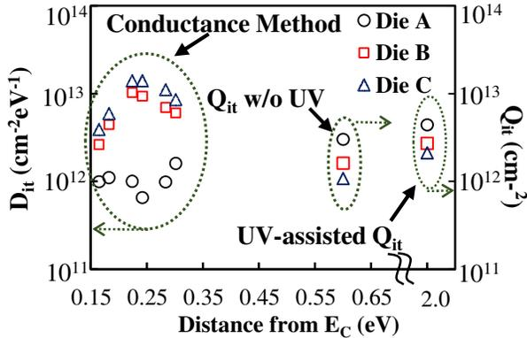
**Fig. 4**  $\text{Al}_2\text{O}_3/\text{AlGaN}$  interface trap density ( $D_{it}$ ) distribution within the AlGaN energy band obtained from conductance method ( $E_T=0.165$  eV to 0.3 eV) and trapped interface charge  $Q_{it}$  from Bi-directional transfer characteristics before ( $E_T=0.6$  eV based on 20s  $I_D$ - $V_G$  sweep rate) and after 10s UV lamp illumination ( $E_T=2$  eV) shown in Table II.
