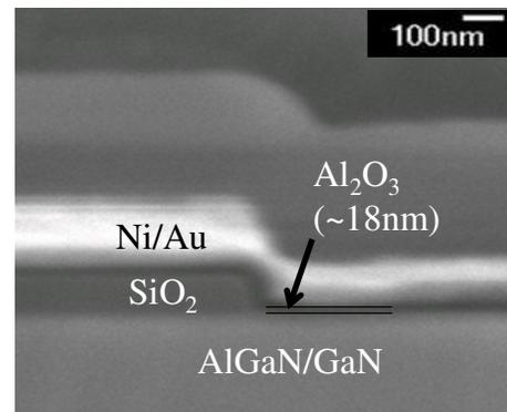
**Fig. 1** (a) Cross-sectional schematics and (b) SEM image of the fabricated device
