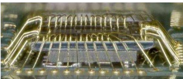
Figure 10. Stacked flip chip + wire bond dies.
