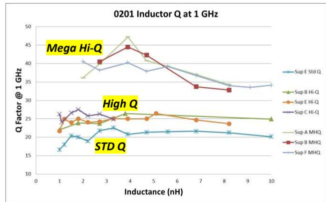
Figure 1. 0201 inductor Q factor at 1GHz.
