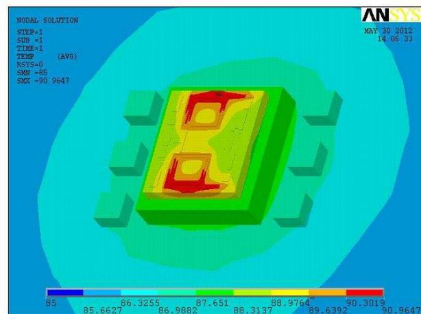
Figure 11. Thermal simulation result for QFN package.
