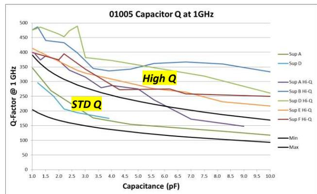
Figure 2. 01005 capacitor Q factor at 1GHz.
