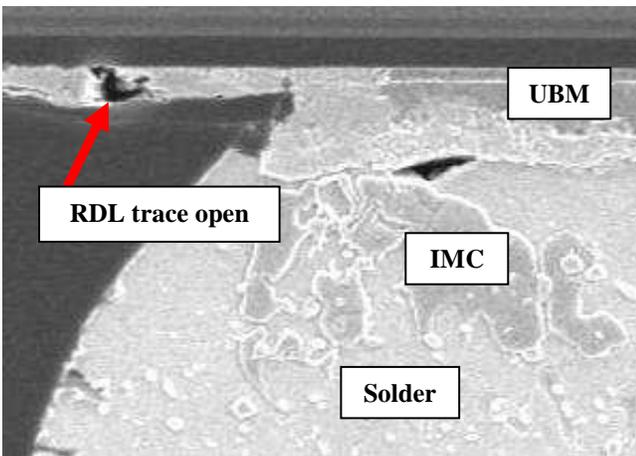
Figure 5. Example of electromigration failure in flip chip solder joint.
