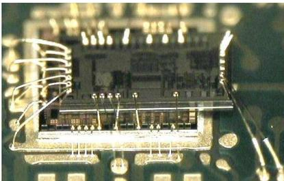
Figure 9. Stacked wire bond dies.
