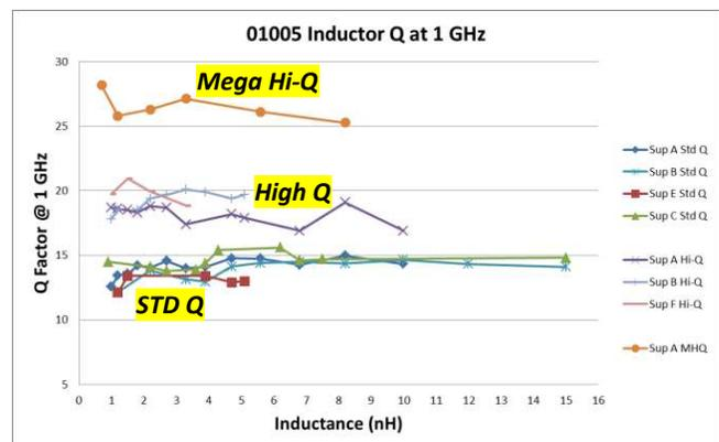
Figure 3. 01005 inductor Q factor at 1 GHz.
