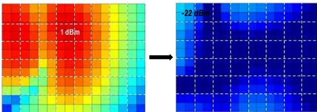
Figure 4. Radiated energy before and after application of module level EMI shielding.
