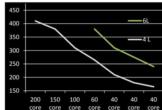
Figure 8. Laminate substrate thickness (um) roadmap.
