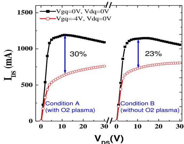
Figure 1. Pulsed I-V characterization of condition A (with O<sub>2</sub> plasma) and condition B (without O<sub>2</sub> plasma) pretreatment prior to 1<sup>st</sup> SiN passivation measurement where Vgq=0V, Vdq=0V, compared with Vgq=-4V, Vdq=0V, pulse width=750nS, and duty cycle=0.1%.
