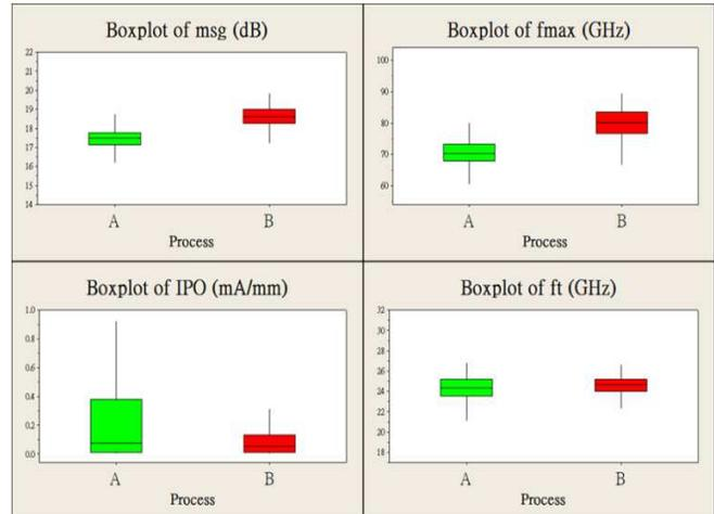
Fig.3. RF PCM chart comparison for condition A (with  $\text{O}_2$  plasma) and condition B (without  $\text{O}_2$  plasma).
