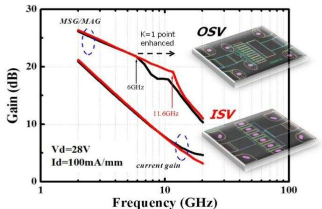
Fig.4. Small-signal gain comparison of the internal source slot via and the outside source circular via.
