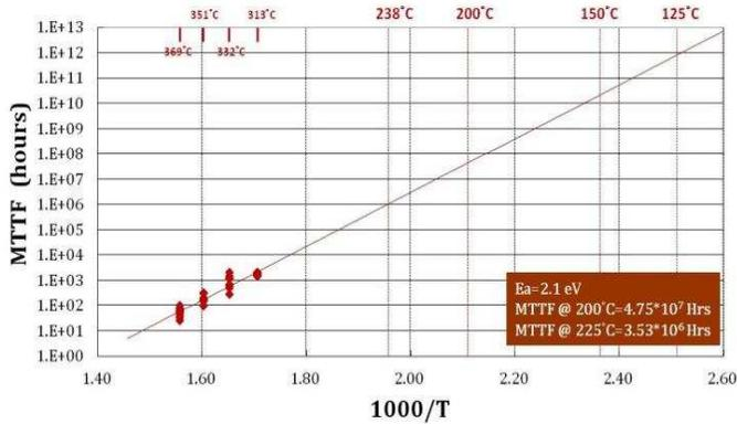
Fig.9. Arrhenius plot of the 0.25µm GaN technology with 20% Idss degradation as the failure criteria.
