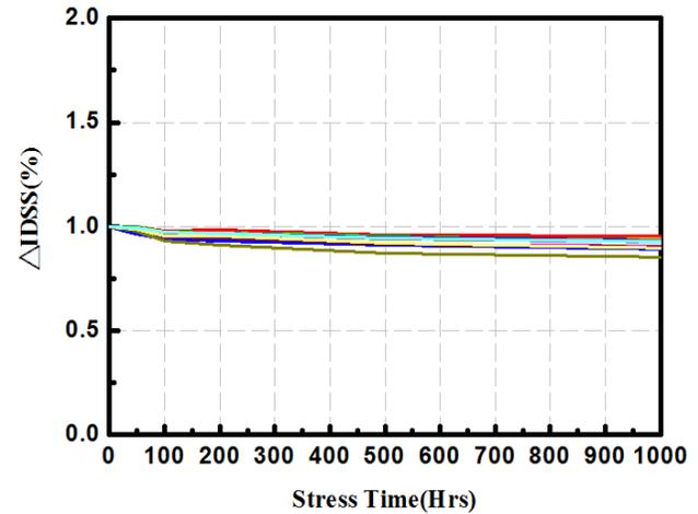
Fig.8. HTRB reliability performance change of the optimized pretreatment (condition B) with IDSS normalized to the initial value. Tests were interrupted in intervals of 50, 100, 200, 500 and 1000 hours.
