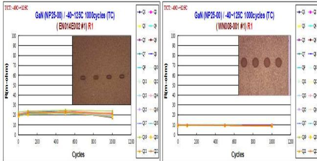
Fig.10. Backside via chain resistance after temperature cycle testing up to 1000cycles comparing a test structure with the 30µm x 60µm slot vias and 85µm diameter circular vias.
