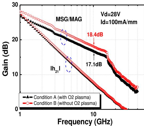
Fig.2. Comparison of small signal of a  $2 \times 125\mu\text{m}$  device performance for the condition A (with  $\text{O}_2$  plasma) and condition B (without  $\text{O}_2$  plasma) pretreatment prior to 1<sup>st</sup> SiN passivation where  $V_d=28\text{V}$  and  $I_d=100\text{mA/mm}$ .
