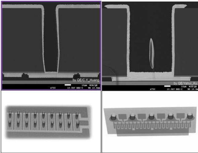
Fig.5. SEM image of the internal source slot via and the outside source circular via
