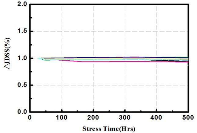
Fig.7. DC HTOL reliability performance change of the optimized pretreatment (condition B) with IDSS normalized to the initial value.
