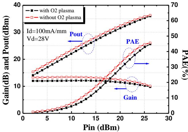
Fig.6. Load-pull comparison of a 10x125μm transistor in continuous-wave operation at 10GHz, with bias points of Vd=28V and Id=100mA/mm, tuned for maximum output power.
