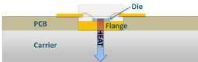
Fig. 3. Cross-section view of multi-level part on PCB and carrier
