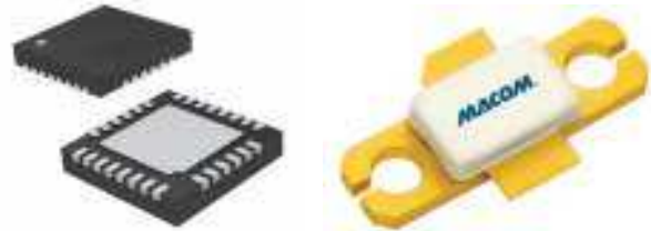
Fig. 1. Co-planar (left) and multi-level (right) package configurations
