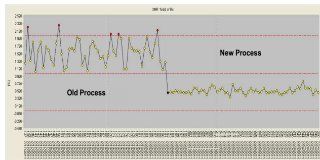
Fig. 5. SPC chart of run average percent standard deviation of sheet resistance. The growth process is switched over to ramp down manipulator temperature earlier in the growth recipe as indicated.
