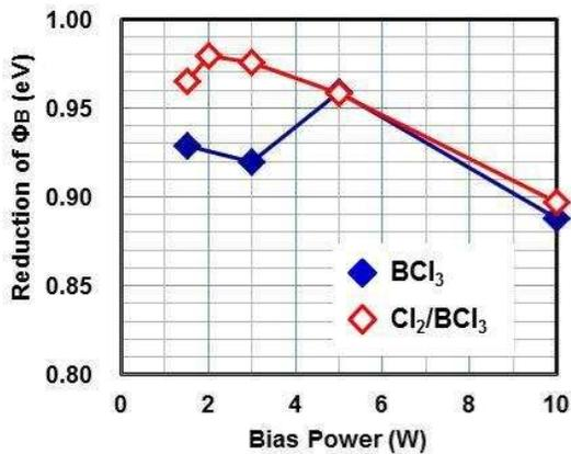
Fig. 6 Comparison of normalized  $\phi_B$  obtained from C-V measurements for  $\text{BCl}_3$  and  $\text{Cl}_2/\text{BCl}_3$  etching.
