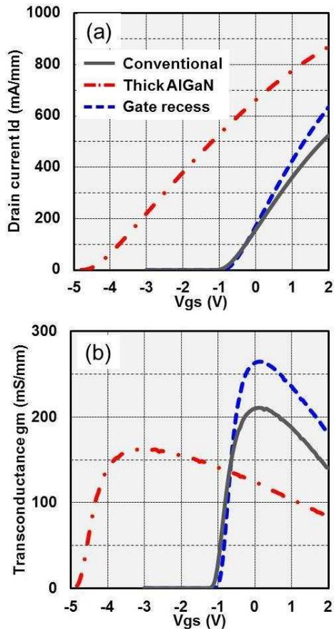
**Fig. 9** Transfer characteristics of fabricated AlGaIn/GaN-HEMTs; (a)  $I_d$ - $V_{gs}$  curves, (b) transconductances.
