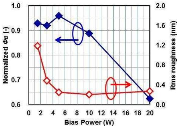
**Fig. 2** Dependence of normalized  $\phi_B$ , calculated from C-V measurements, and RMS roughness on bias power for  $\text{BCl}_3$  etching.
