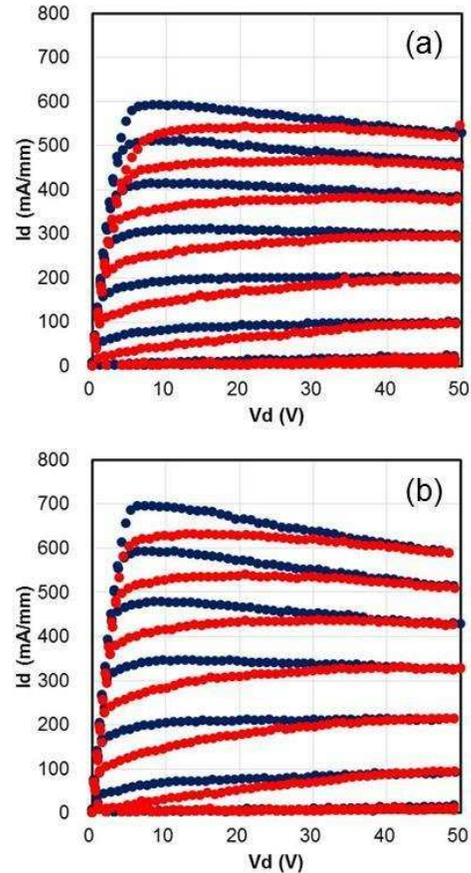
**Fig. 10** Pulsed I-V curves of fabricated AlGaIn/GaN-HEMTs; (a) conventional, (b) gate recess structure.  $V_{gs}$  was stepped from -3 V to +2 V with a 0.5 V step. The bias stress was  $V_{gs} = -3$  V and  $V_{ds} = 50$  V.
