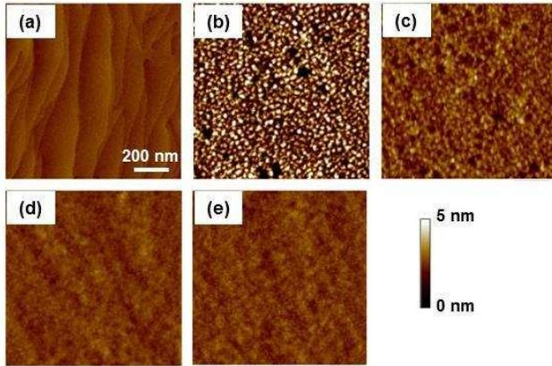
**Fig. 1** AFM images of GaN surface etched by  $\text{BCl}_3$  etching process ;(a)as-grown, (b)bias power 1.5 W, (c)bias power 3 W, (d)bias power 10 W, (e)bias power 20 W.
