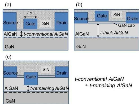
Fig. 8 Schematic of fabricated AlGaIn/GaN-HEMTs; (a) conventional, (b) thick AlGaIn epitaxial layer, (c) gate recess structure.
