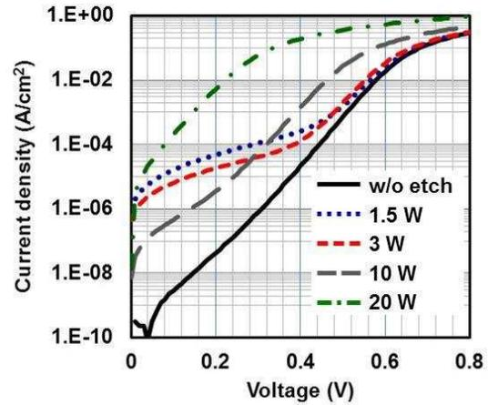
**Fig. 3** Current-voltage characteristics of SBDs fabricated on the  $\text{BCl}_3$  etched surface.
