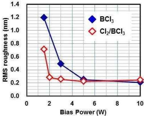
Fig. 5 Comparison of RMS roughness obtained from  $\text{BCl}_3$  and  $\text{Cl}_2/\text{BCl}_3$  etching.
