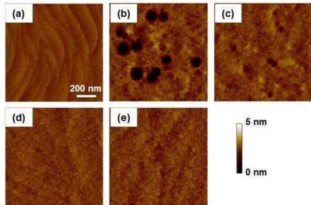
**Fig. 4** AFM images of  $\text{Cl}_2/\text{BCl}_3$  etched GaN surface; (a)as-grown, (b)bias power 1.5 W, (c)bias power 2 W, (d)bias power 5 W, (e)bias power 10 W.
