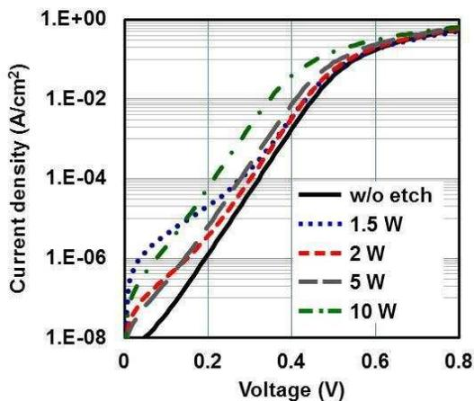
Fig. 7 Current-voltage characteristics of SBDs fabricated on the  $\text{Cl}_2/\text{BCl}_3$  etched surface.
