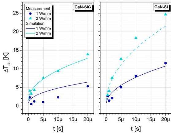
**Figure 8:** Comparison of measured and simulated  $\Delta T_{ch}$  for power dissipation of 1 and 2 W/mm, representing the linear region of I-V characteristics, for Si and SiC substrates.
