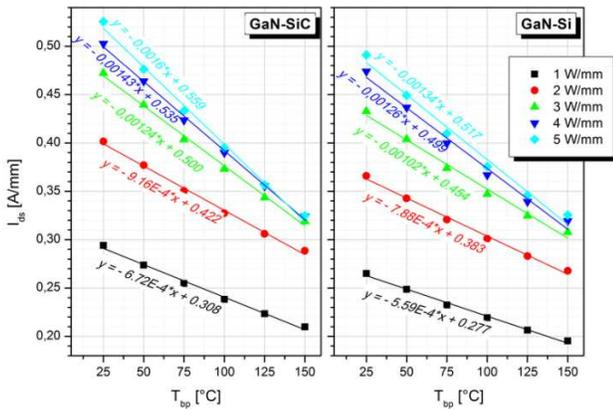
Figure 3:  $I_{ds}(T)$  extracted at  $t = 0.5$   $\mu$ s for varying power conditions on Si and SiC substrates. Approximation by linear equations is presented by lines.
