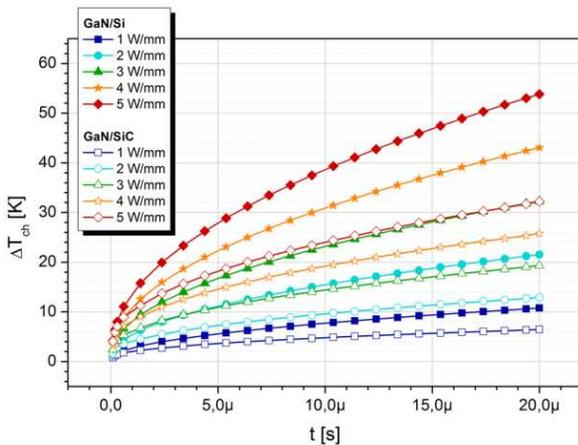
**Figure 7: Delta of channel temperature ( $T_{ch}-T_{bp}$ ) depending on time simulated with ANSYS for power dissipation of 1...5 W/mm for Si and SiC substrates.**
