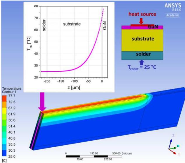
**Figure 6: Temperature distribution simulated with ANSYS for power condition of 5 W/mm on Si substrate after pulse length of 20  $\mu$ s. Inset:  $T_{ch}$  along marked z coordinate.**
