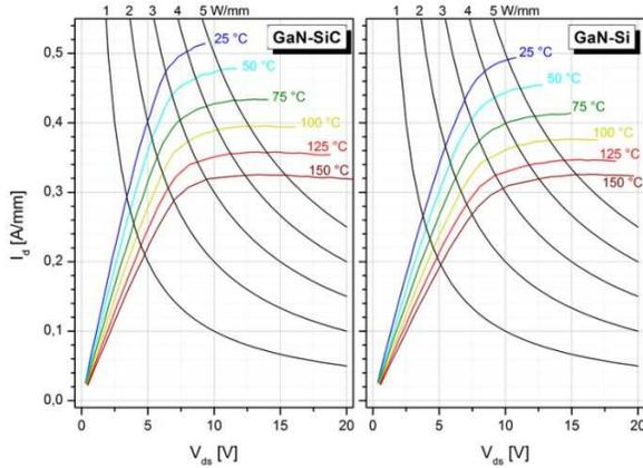
Figure 2: Pulsed (at 0.5  $\mu$ s)  $I_{ds}$ - $V_{ds}$  characteristics measured at  $V_{gs} = +4.4$  V for GaN-on-SiC and  $V_{gs} = +4.6$  V for GaN-on-Si at base plate temperatures varying from 25 °C to 150 °C.
