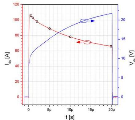
Figure 1: Exsample of pulsed IV characterisation of large periphery devices fabricated on Si substrates, pulse duration 20  $\mu\text{s}$ . Circular marks show extraction points of time regions.
