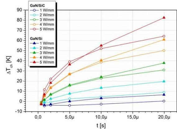
Figure 5: Delta of channel temperature ( $T_{ch} - T_{bp}$ ) depending on time calculated from figure 4 for power dissipation of 1...5 W/mm for Si and SiC substrates.
