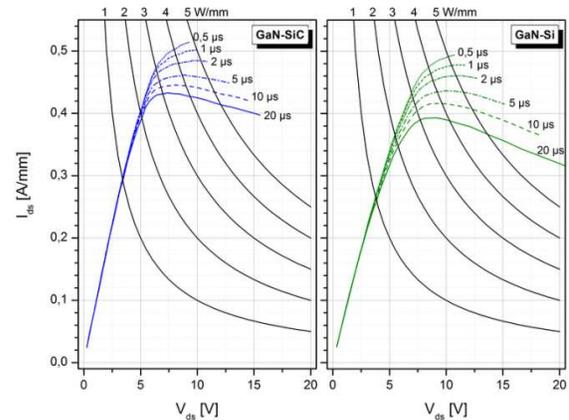
Figure 4: Pulsed  $I_{ds}$ - $V_{ds}$  characteristics measured at  $V_{gs} = +4.4$  V for GaN-on-SiC and  $V_{gs} = +4.6$  V for GaN-on-Si extracted at time points 0.5...20  $\mu$ s at base plate temperature of 25 °C.
