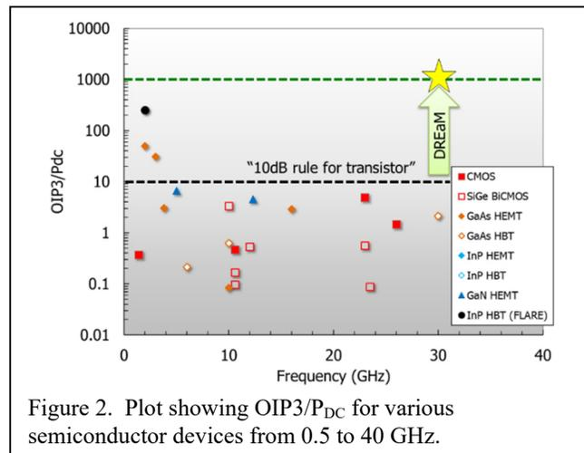
Figure 2. Plot showing  $OIP3/P_{DC}$  for various semiconductor devices from 0.5 to 40 GHz.
