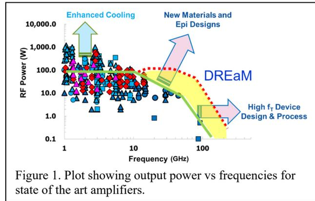
Figure 1. Plot showing output power vs frequencies for state of the art amplifiers.
