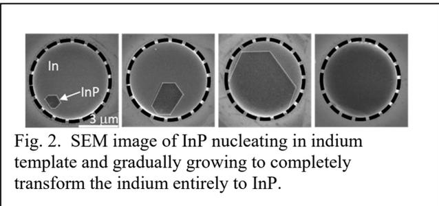
Fig. 2. SEM image of InP nucleating in indium template and gradually growing to completely transform the indium entirely to InP.
