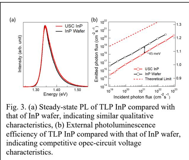
Fig. 3. (a) Steady-state PL of TLP InP compared with that of InP wafer, indicating similar qualitative characteristics, (b) External photoluminescence efficiency of TLP InP compared with that of InP wafer, indicating competitive open-circuit voltage characteristics.
