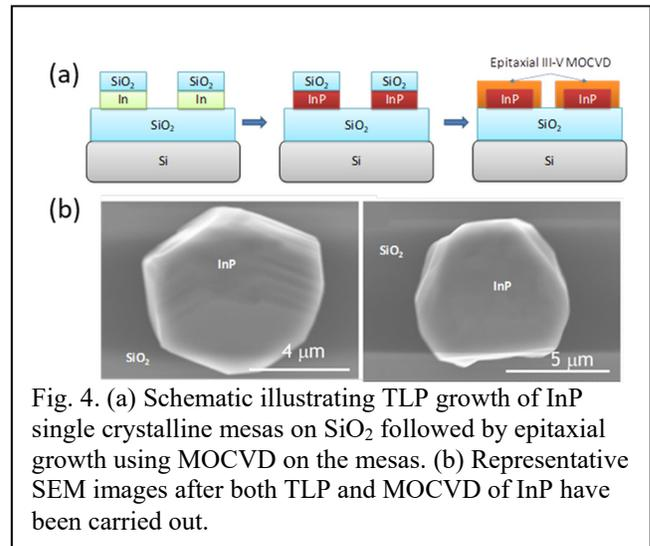
Fig. 4. (a) Schematic illustrating TLP growth of InP single crystalline mesas on  $\text{SiO}_2$  followed by epitaxial growth using MOCVD on the mesas. (b) Representative SEM images after both TLP and MOCVD of InP have been carried out.
