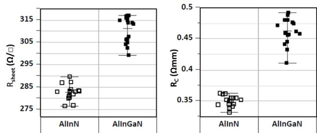
Fig. 4. Sheet resistance  $R_{\text{sheet}}$  and contact resistance  $R_c$  extracted from TLM measurements for samples with AlInN and AlInGaN barriers.
