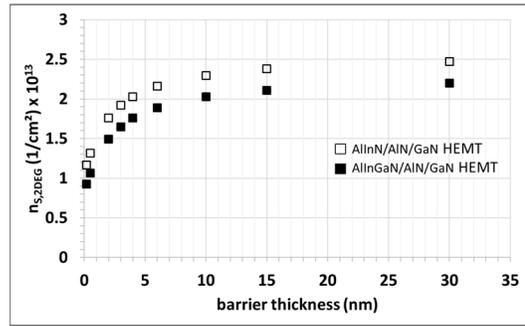
Fig. 3. Density of electrons in the 2DEG as a function of barrier thickness for ternary and quaternary structures.
