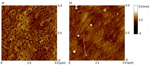
Fig. 1.  $5 \times 5 \mu\text{m}^2$  AFM image of a) AlInN/AlN/GaN HEMT structure and b) AlInGaN/AlN/GaN HEMT structure.
