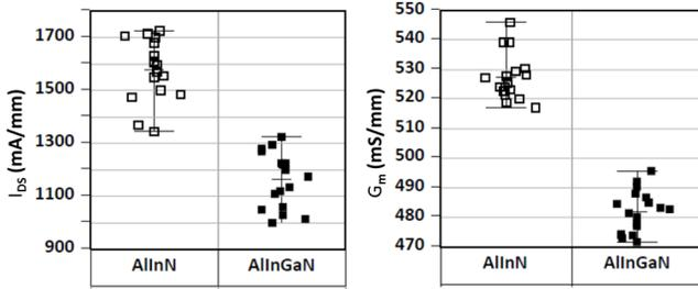
Fig. 5. Maximum drain saturation current  $I_{DS}$  and maximum transconductance  $G_m$  measured at  $V_{GS} = -2$  V and  $V_{DS} = 7$  V.
