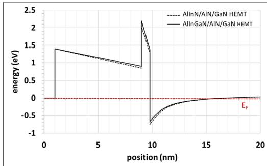
Fig. 2. Conduction band profile of the AlInN/AlN/GaN HEMT (dotted line) and of the AlInGaN/AlN/GaN HEMT (solid line).
