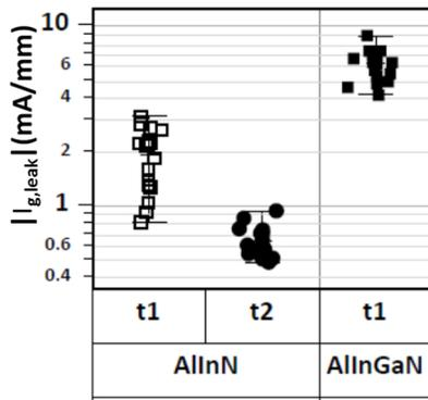
Fig. 6. Leakage current  $I_{g,leak}$  for ternary and quaternary barrier material for different barrier thickness  $t1$  and  $t2$  at  $V_{DS} = 7$  V.
