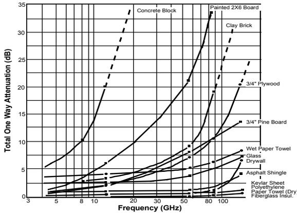
Figure 3. Attenuation through different mediums as a function of frequency [3].
