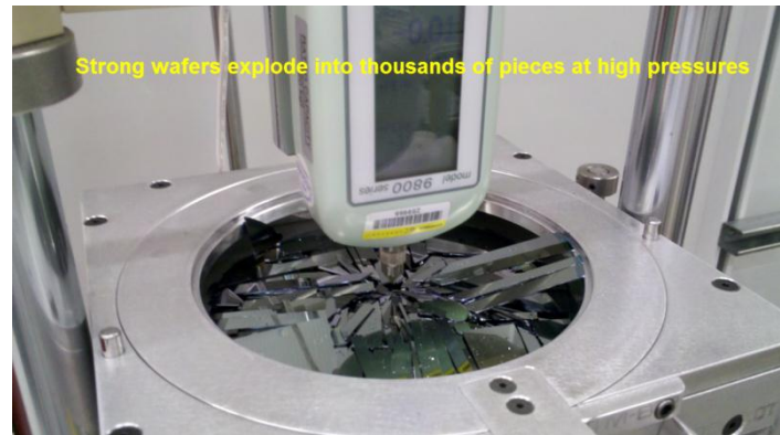
Fig.4: Different types of breaks, weak and strong wafers.
