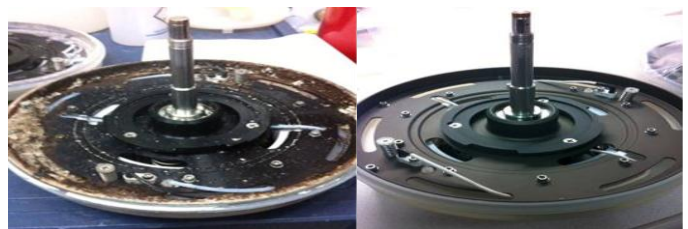
Figure 4. Plating rotor before and after “in house” repair.
