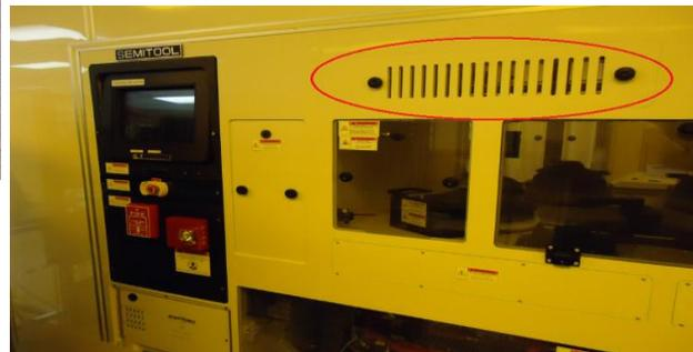
Figure 9. Plating cabinet louvers to block air flow (circled).
