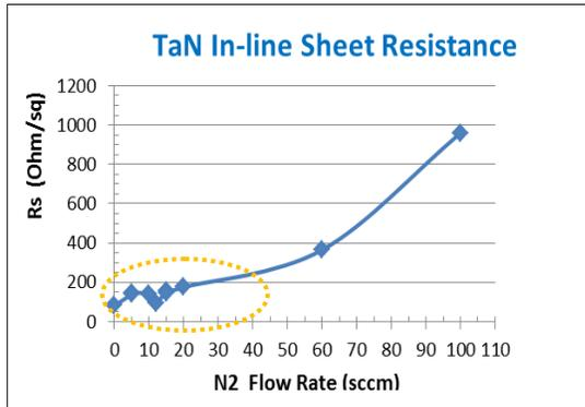
Figure 1 (b): TaNx Film Sheet Resistance as a function of N2 flow.
