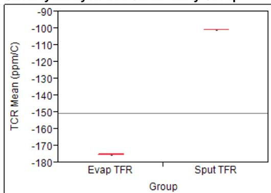
Figure5: Quantile plots of sputtered vs. evaporated TFR TCR.
