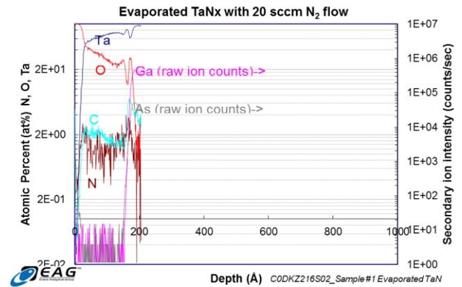
Figure 4 (b): SIMS of evaporated TaNx film with 20 sccm of N<sub>2</sub> flow showing N<sub>2</sub> peak as well as O<sub>2</sub> peak.
