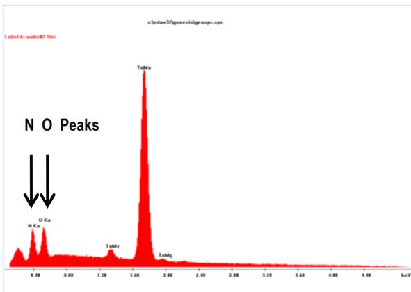
Figure 3: EDX of evaporated TaNx film showing N<sub>2</sub> peak as well as O<sub>2</sub> peak.
