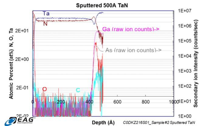
Figure 4 (a): SIMS of sputtered TaNx film showing N<sub>2</sub> peak and low level of O<sub>2</sub>.
