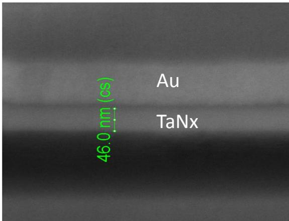
Figure 2: FIB cross section of an approximately 500 angstroms evaporated TaNx film.
