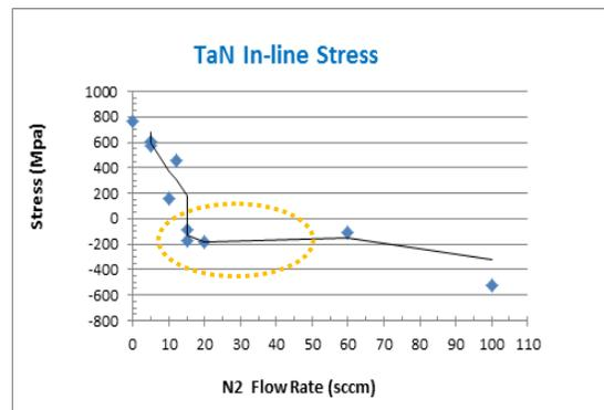
Figure 1 (a): TaNx Film Stress as a function of  $N_2$  flow.
