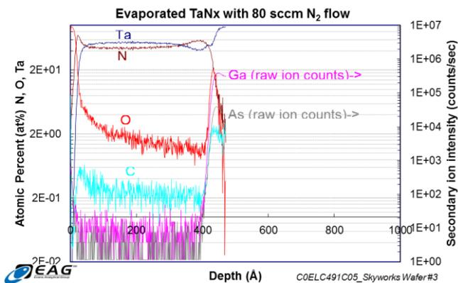
Figure 4 (c) SIMS of evaporated TaNx film with 80 sccm of N<sub>2</sub> flow showing N<sub>2</sub> peak as well as O<sub>2</sub> peak. Courtesy of Chris Sheppard, Skyworks, Woburn.
