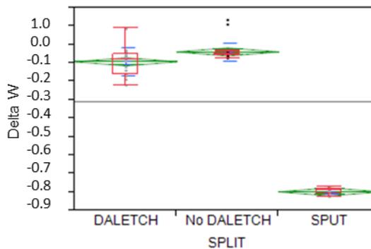
Figure 6: Width correction factor, delta w comparison of standard sputtered vs. evaporated film, ran with photo mask corrected for standard sputter DAL process with 0.8µm process bias.
