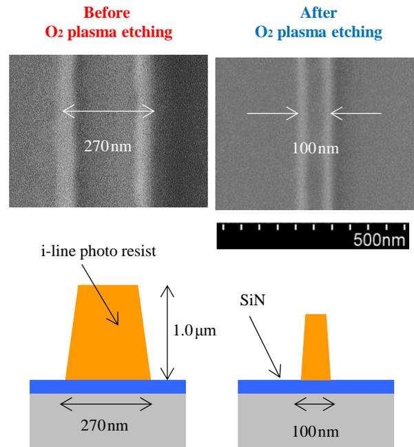
Fig. 2 SEM upper views and schematic cross-sectional images of the resist pattern before and after the O<sub>2</sub> plasma.
