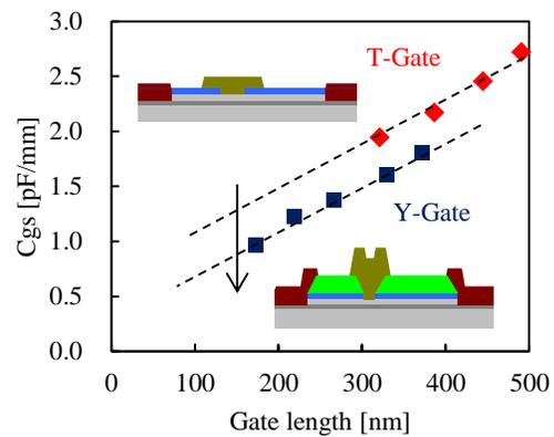
Fig. 10  $C_{gs}$  comparison between T-gate and Y-gate of the InAlN/GaN HEMTs.
