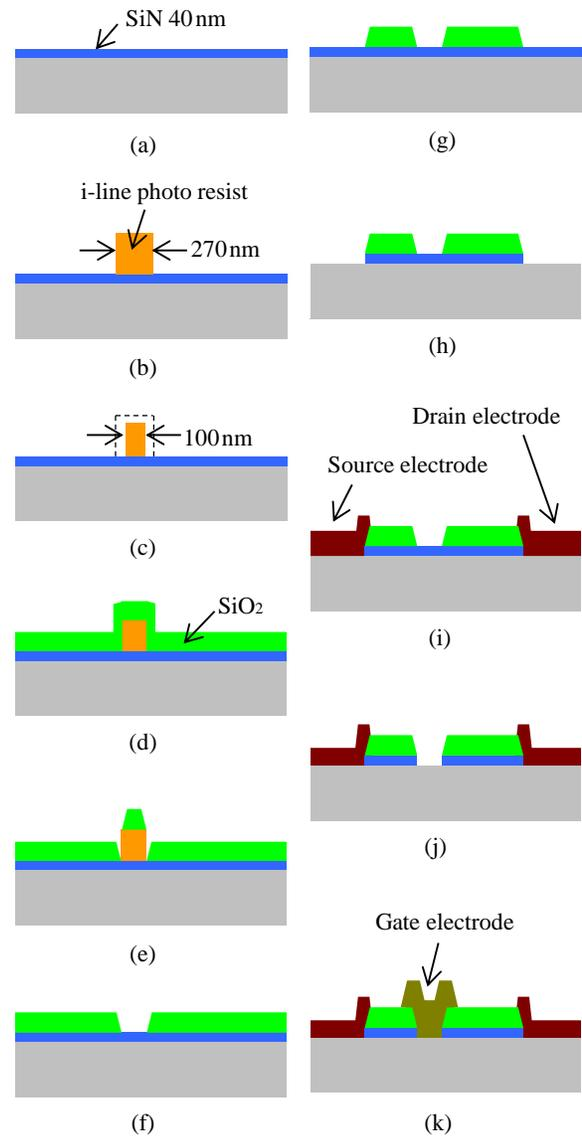
Fig. 1 Y-gate process flow using an i-line stepper
