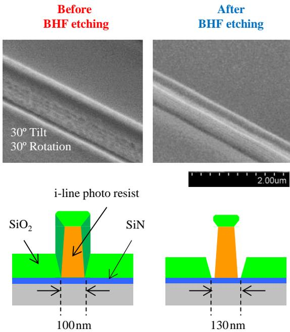
Fig. 4 SEM bird's-eye views and schematic cross-sectional images of the resist pattern before and after the BHF etching in collimated sputtering method.
