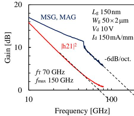
Fig. 9 Small-signal frequency response of the InAlN/GaN HEMT.
