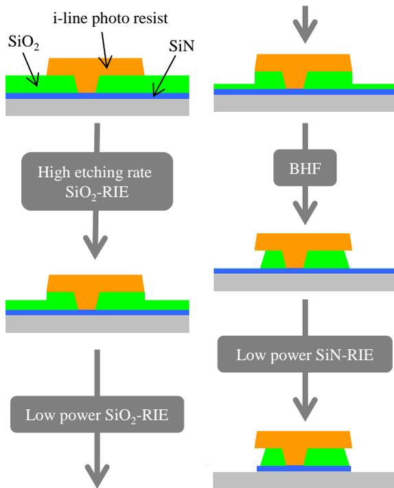
Fig. 5 Process flow of four steps SiO<sub>2</sub>/SiN opening.
