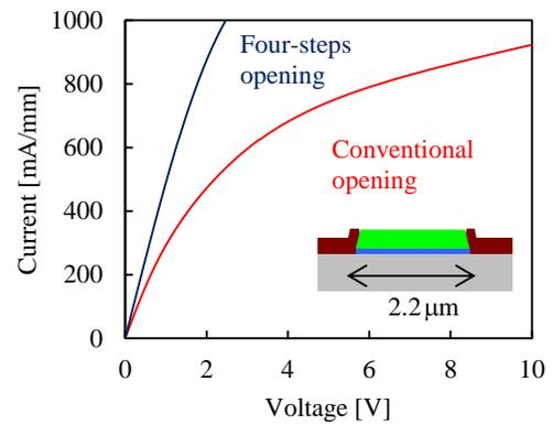
Fig. 6  $I$ - $V$  characteristics of different SiO<sub>2</sub>/SiN opening methods.
