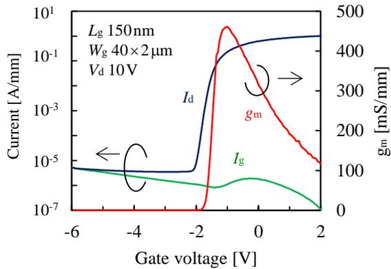
(b) Transconductance and  $I_d$ ,  $I_g$ - $V_g$  characteristics.
