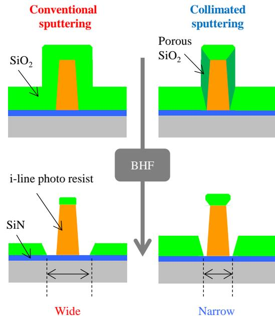
Fig. 3 Comparison the sputtering methods. Schematic cross-sectional images of the resist pattern before and after the BHF etching.
