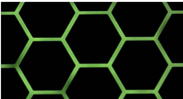
Figure 8. Hexagonal die produced by plasma-based singulation viewed by backlit illumination. Die are still on tape. Die dimensions are approximately 150µm.
