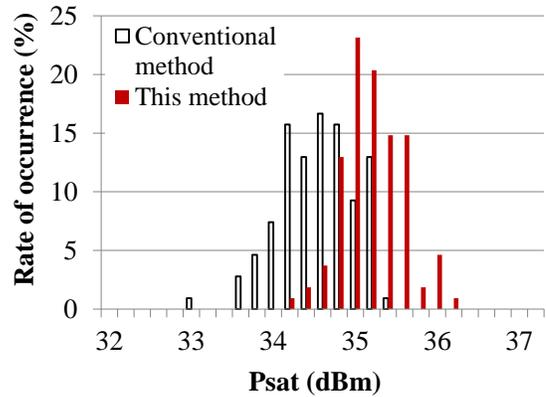
Figure 9. Comparison of the Psat in distribution (Simulation)
