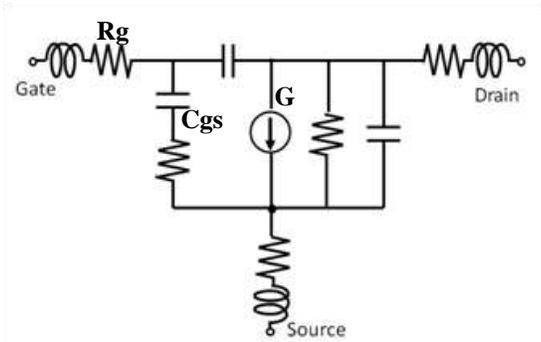
Figure 5. The nonlinear equivalent circuit model of a transistor (Angelov Model)
