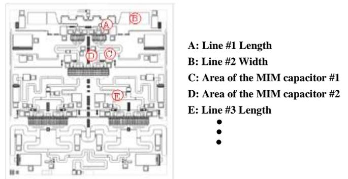
Figure 4. The circuit layout of the power amplifier
