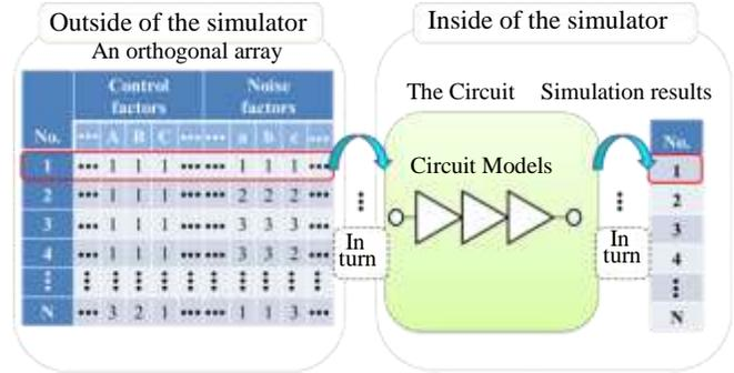
Figure 3. Simulation technique using the orthogonal array
