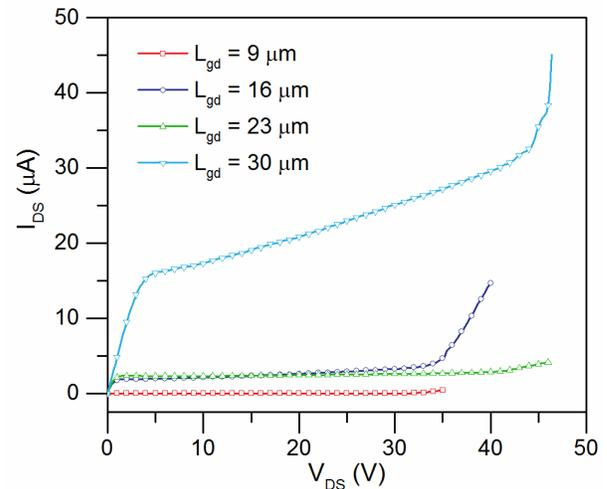
Fig. 4. Breakdown characteristics of the ZnO SGTFTs with varying gate-to-drain spacing at zero gate bias.
