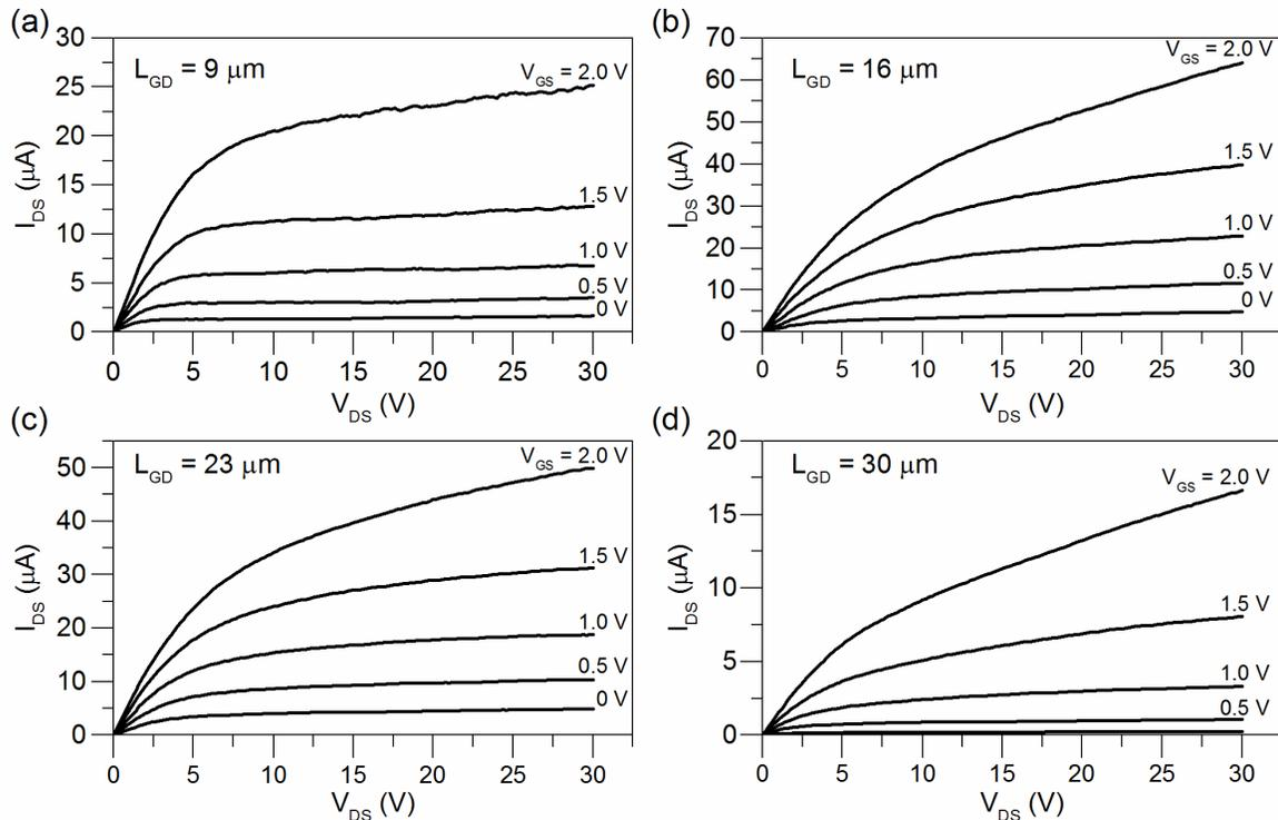
Fig. 2. Output Characteristics of the ZnO SGTFT with a gate-to-drain spacing of (a) 9  $\mu\text{m}$ , (b) 16  $\mu\text{m}$ , (c) 23  $\mu\text{m}$ , and (d) 30  $\mu\text{m}$ .
