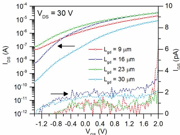
Fig. 3. Left (solid lines + symbols): Transfer characteristics of the ZnO SGTFTs. Right (dashed lines): Gate leakage characteristics of the ZnO SGTFTs.
