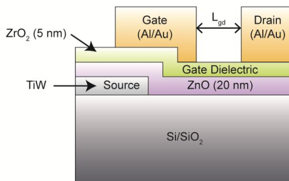
Fig. 1. Cross-section schematic image of the ZnO SGTFT.
