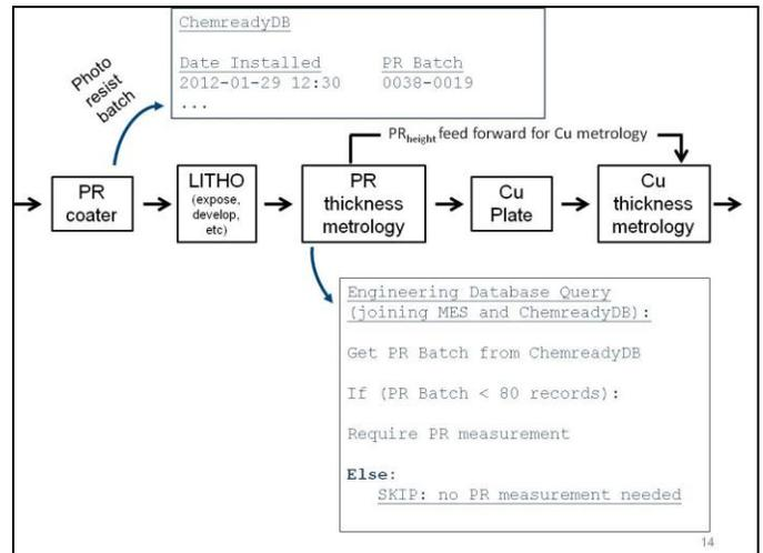
There are two main components to the system. The first component is that all PR batches loaded onto the coaters are logged in our internal tool-chemical database (called “ChemreadyDB”). Secondly, at the point of PR<sub>height</sub> measurement, the operator scans the production lot ID into a web-based data entry form. The host program then queries
