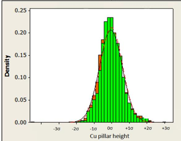
Green = Cu<sub>height</sub> distribution from measuring PR on all wafers.
