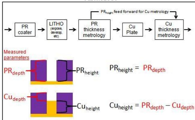
In the early stages of our Cu pillar process when PR thickness control was relatively poor ( $1\sigma = 1.7\mu m$ ),  $PR_{height}$  measurements were taken for every wafer in every lot. On average, the combined processing and queue time for each lot
