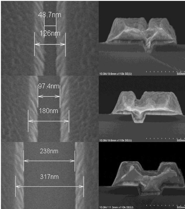
Figure 4. SEM images of different openings in SiN<sub>x</sub> (top views, left) and cross sections of gates fabricated in corresponding trenches (right).
