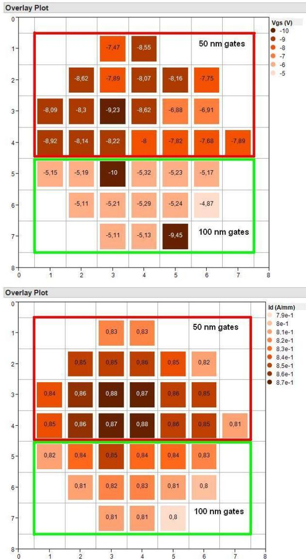
Figure 8.  $I_{DS,max}$  (top) and  $V_{th}$  (bottom) distribution over wafer area for  $2 \times 50\text{-}\mu\text{m}$  transistors with  $L_g = 50\text{ nm}$  and  $L_g = 100\text{ nm}$
