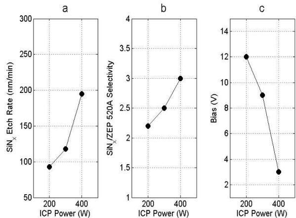
Figure 3. Dependencies of a)  $\text{SiN}_x$  etch rate, b)  $\text{SiN}_x$ /mask selectivity and c) bias level on ICP power level for a  $\text{CHF}_3/\text{SF}_6$  flow ratio of 15.
