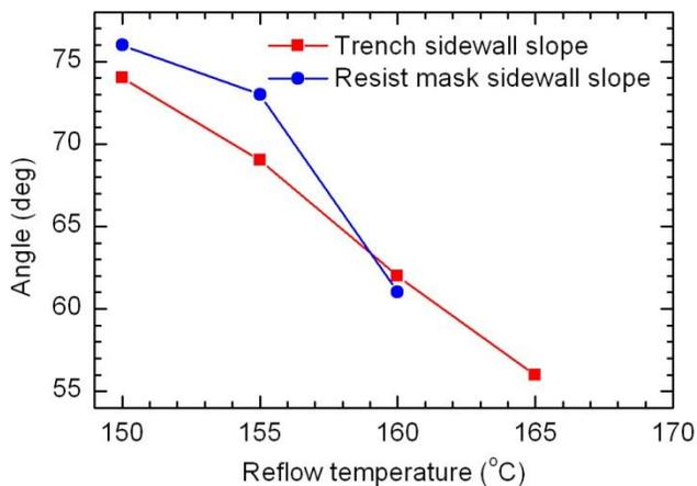
Figure 2. Angle of sidewall slopes versus reflow temperature.
