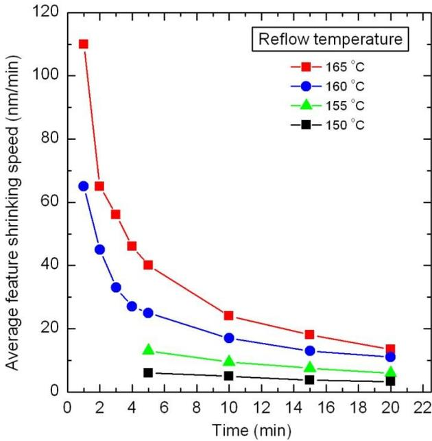
Figure 1. Average feature shrinking speed versus process time for various temperatures.
