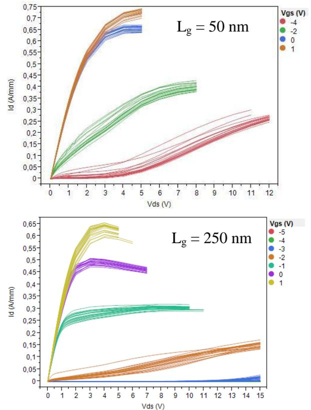
Figure 7. DC output characteristics of  $2 \times 125$ - $\mu\text{m}$  transistors with  $L_g=50$ nm, 100 nm and 250 nm
