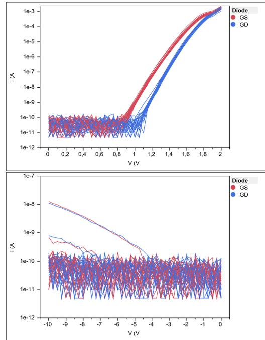
Figure 6. Diode characteristics for forward (top) and backward (bottom) bias conditions (gate-source and gate-drain diodes have been measured)
