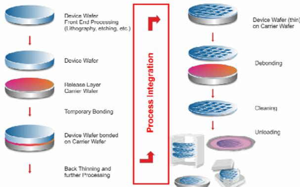
**Figure 1.** Generic Temporary Bonding / Debonding Process Flow
