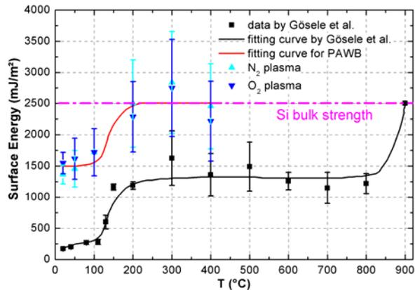
Figure 3. Surface energy of bonded Si/SiO<sub>2</sub> wafer pairs annealed at various temperatures for high temperature oxide bonding and plasma activated wafer bonding using N<sub>2</sub> respectively O<sub>2</sub> plasma. The maximum bond strength of 2.5J/m<sup>2</sup> is indicated by the dashed-dotted horizontal line. Data for high temperature process was taken from Ref. [3]
