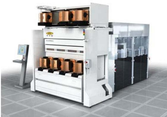
**Figure 2.** This production platform for temporary bonding and debonding can accommodate up to 9 process modules.
