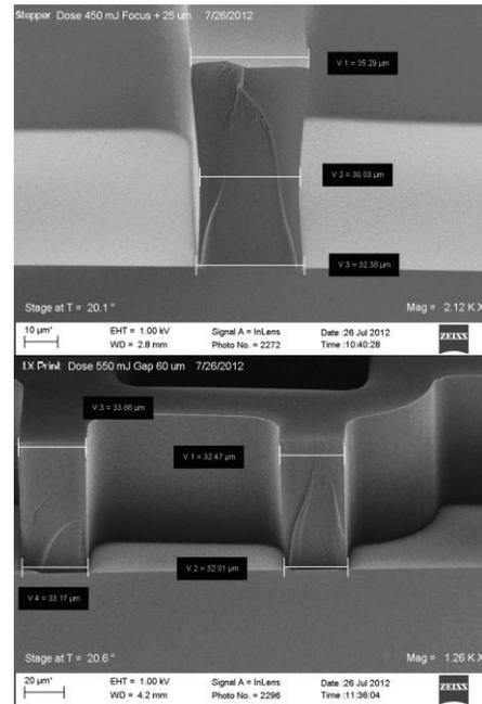
Figure 3: SU8 Structure Cross Section Profiles
