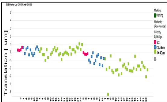
Figure 5: Alignment Translation Error of SU8 Structures Exposed on a 5X Stepper vs. a 1X Proximity Printer
