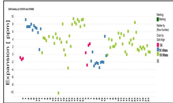
Figure 6: Alignment Expansion Error of SU8 Structures Exposed on a 5X Stepper vs. a 1X Proximity Printer
