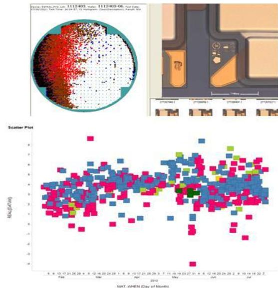
Figure 2: Alignment shift from Mask Touching
