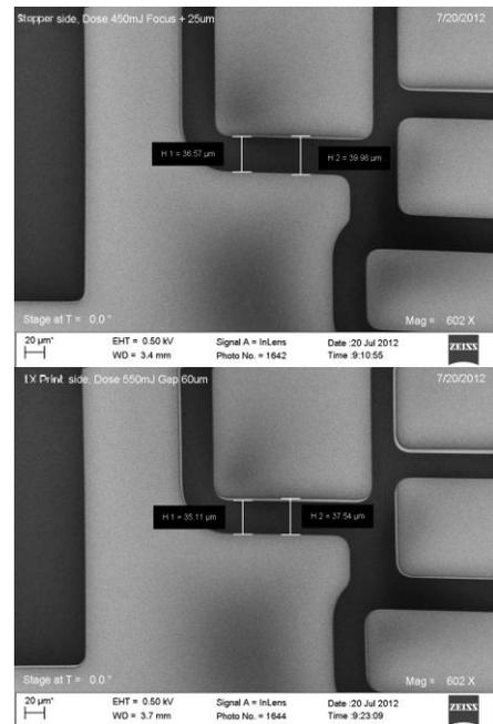
Figure 4: SEM CD Comparison on Pilot Wafers
