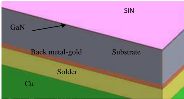
Fig. 1a. Close-up of chip/package
