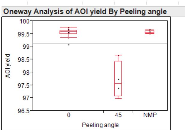
Fig.2a AOI yield for different peeling orientation
