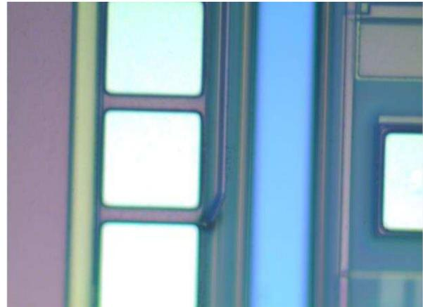
Fig.3 Metal wire is peeling from polyimide surface
