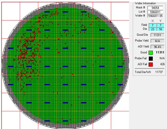
Fig. 2b AOI yield loss due to the metal damage
