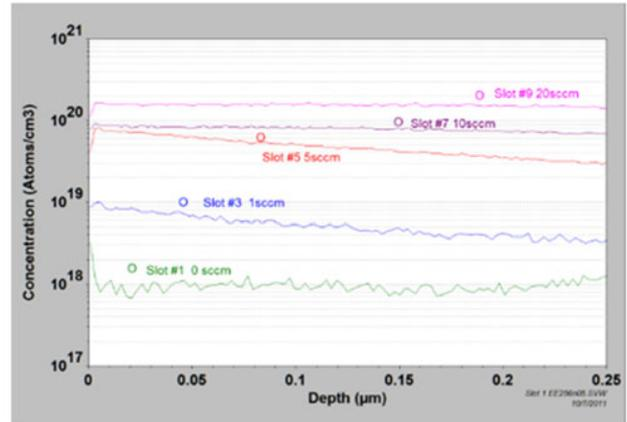
Fig. 5. SIMS analysis of oxygen level of films with different gas contamination during sputtering.
