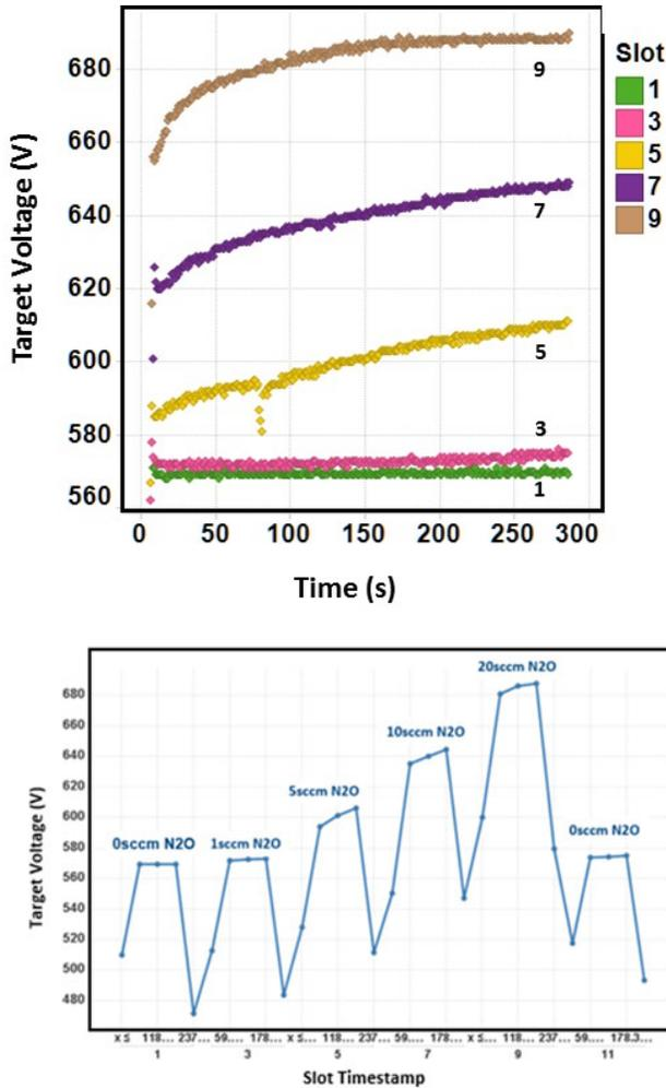
Fig. 4. Experiment result of target voltage of wafers with different level of gas contamination during Pt sputtering.
