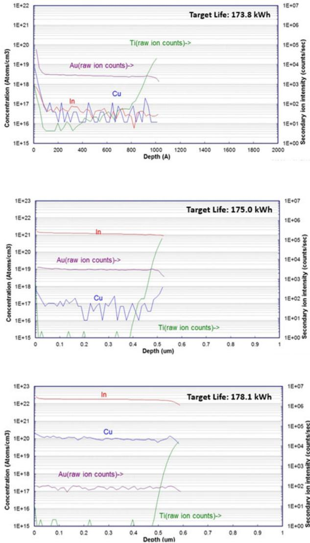
Fig. 2. SIMS analysis of deposited films at target life of 173.8 kWh, 175 kWh and 178.1 kWh.
