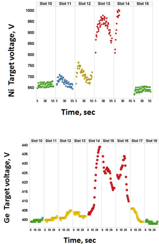
Fig. 3. Target voltage shift of Ni and Ge target during a process gas contamination event.
