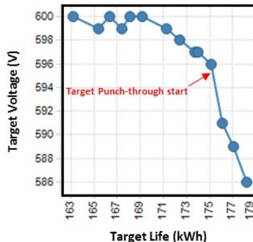
Fig. 1. Target voltage vs Target life of an Au target during target punch-through.
