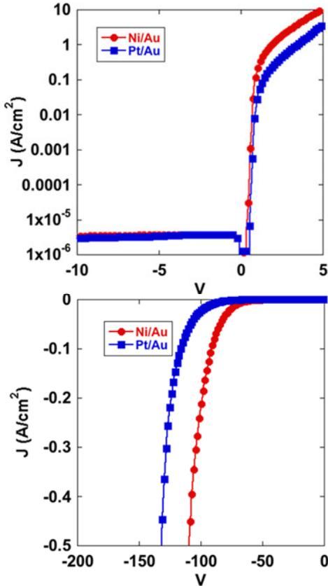
Fig. 4. Quasi-vertical Schottky barrier diode I-V characteristics of 5 μm GaN templates on 6-inch QST™.
