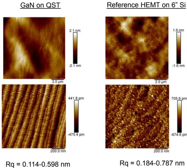
Fig. 2. AFM images comparing GaN on 150 mm QST™ to GaN HEMTs grown on 150 mm Si.
