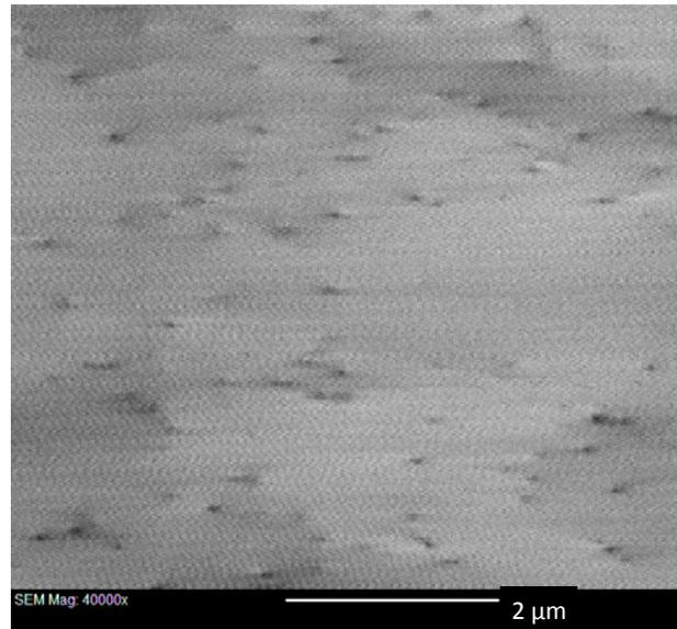
Fig. 3. Example electron channeling contrast image of 16 μm thick GaN grown on 150 mm QST™ substrate by MOCVD.
