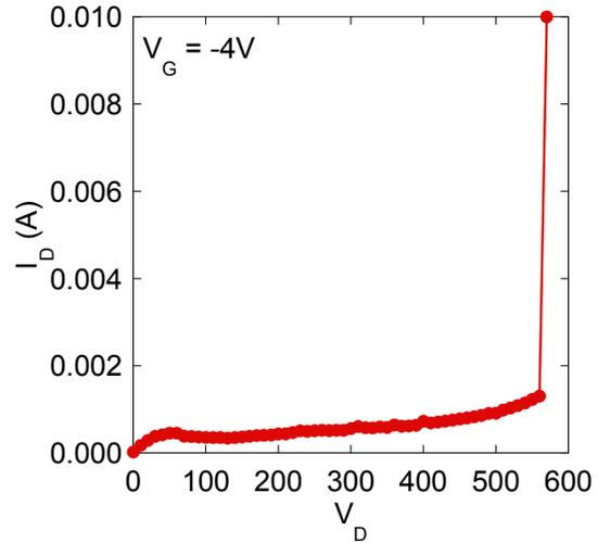
Fig. 7. AlGaIn/GaN HEMT on 150 mm QST™ substrate blocking characteristic.
