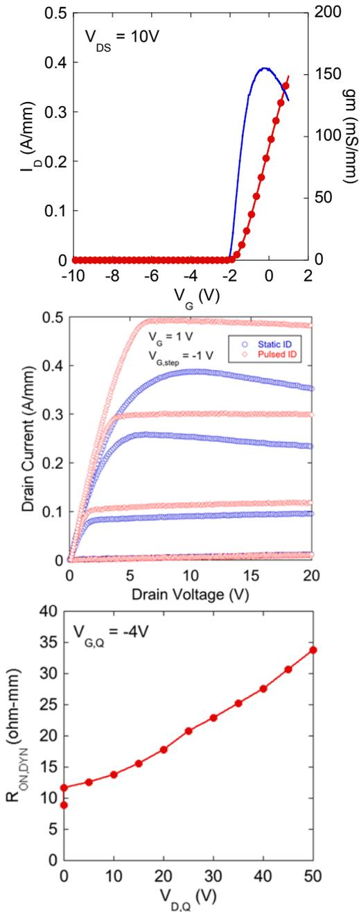
Fig. 6. HEMT transfer, transconductance, pulsed (quiescent point:  $V_{G,Q} = 0$  V,  $V_{D,Q} = 0$  V, which represents the lowest point on the  $R_{ON,DYN}$  vs.  $V_{D,Q}$  curve at  $V_{D,Q} = 0$ ) and static current-voltage, and dynamic on-resistance curves.
