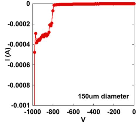
Fig. 5. Reverse breakdown of Schottky barrier diode on thick (~16 μm) GaN on 150 mm QST™ substrate.
