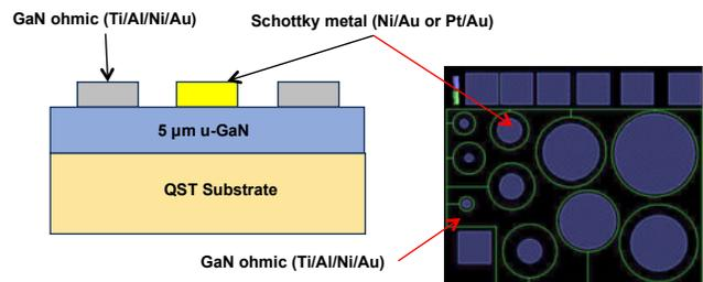
Fig. 1. Schematic cross-section of annular GaN Schottky diodes and the corresponding plan view of the mask.
