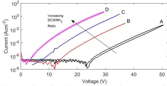
Fig. 1. Leakage through LPCVD SiN<sub>x</sub> layer measured on 100 μm by 100 μm test structure.
