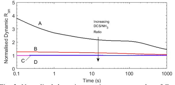
Fig. 3. Normalised dynamic on-resistance measured on fully processed AlGaIn/GaN HEMTs after 1000s off-state stress ( $V_{GS} = -5V$ ,  $V_{DS} = 100V$ ).
