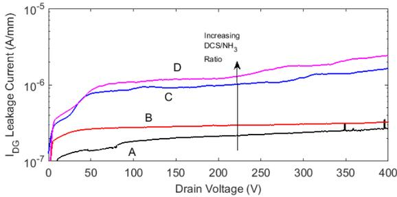
Fig. 2. Off-state drain leakage ( $V_{GS} = -5V$ ) measured on fully processed AlGaIn/GaN HEMTs.
