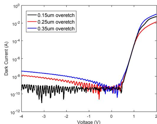
Fig. 4. Dark current of  $20\ \mu\text{m}$  aperture PIN photodiodes with various mesa overetch depths.
