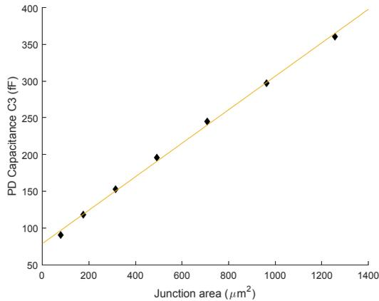
Fig. 6. Photodiode junction capacitance vs. aperture area.
