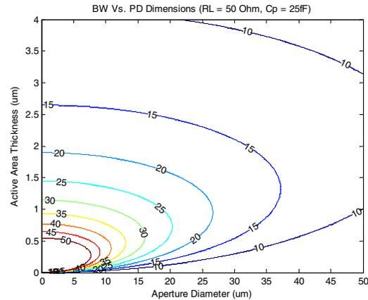
Fig. 1 (Color online). Design curves showing the bandwidth of the PIN photodiode as a function of intrinsic region thickness and aperture diameter  $A$  combined load resistance of 50  $\Omega$  and a parasitic capacitance of 25 fF were assumed.
