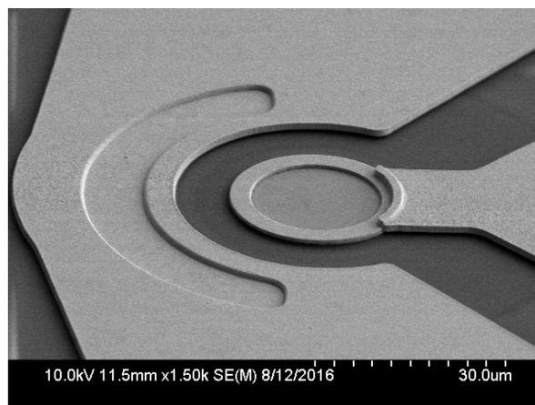
Fig. 3. Completed PIN photodiode after planarization, via opening, and top metal deposition.
