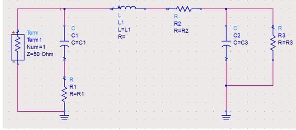
Fig. 5. Small-signal model of a PIN photodiode.
