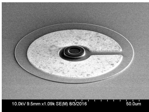
Fig. 2. PIN photodiode before planarization using BCB.
