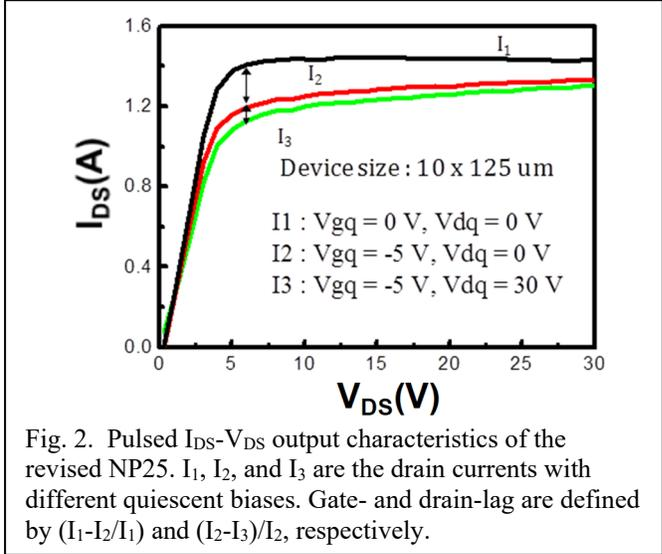
respectively. The gate- and drain-lag are mainly reduced by changes in the gate module including gate metal stack, surface pretreatment prior to gate metallization and by changes to the epitaxial layer structure and growth.
