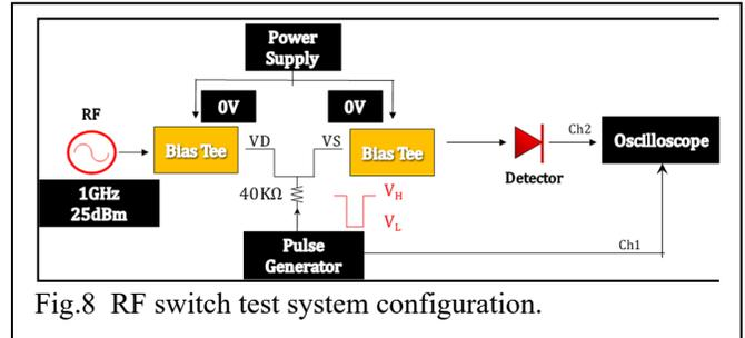
Fig.8 RF switch test system configuration.
