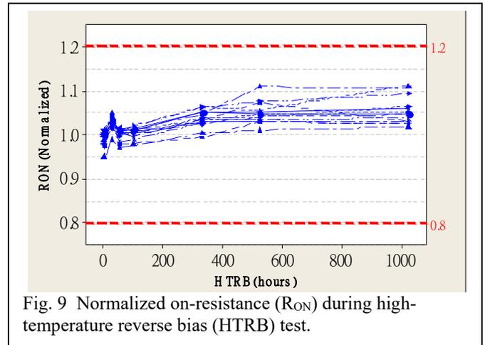
Fig. 9 Normalized on-resistance ( $R_{ON}$ ) during high-temperature reverse bias (HTRB) test.
