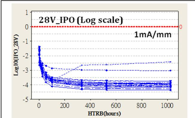
Fig. 7. Normalized off-state 3-terminal drain leakage current ( $28V_{IPO}$ ) at  $V_{GS}=-8V$  and  $V_{DS}=28V$  during high temperature reverse bias (HTRB) test.
