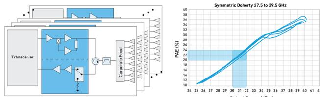
Fig. 8. mmWave GaN Doherty and Low-Noise Switch-LNA Front-End Module
