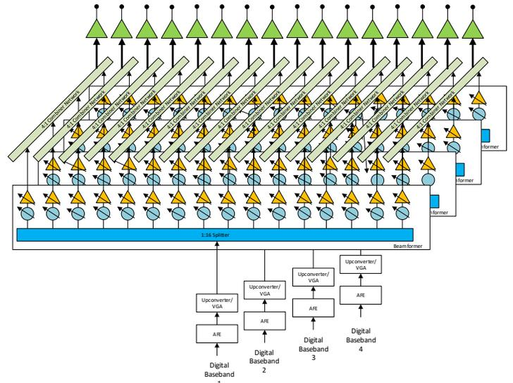
Fig. 1. Fully-connected Shared-aperture hybrid beamformer
