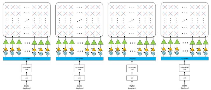
Fig. 2. Sub-array Panned hybrid beamformer
