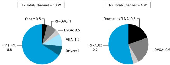
Fig. 7. Power Dissipation Budget of TX and RX Chains
