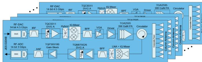
Fig. 6. High Power All-Digital Beamforming AAS – Using Today's Off-the-shelf Components
