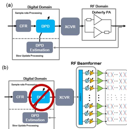
Fig. 5. (a) 1:1 mapping of baseband DPD and Doherty PA; (b) shows that DPD is not effective in a 1:N analog beamforming configuration
