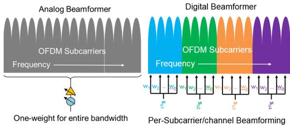
Fig. 3. Hybrid beamforming doesn't allow the frequency to be subdivided to different users during a timeslot
