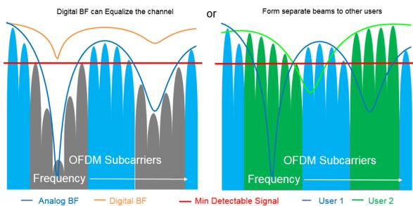
Fig. 4. In frequency selective conditions, all-digital beamforming systems can fully utilize the channel
