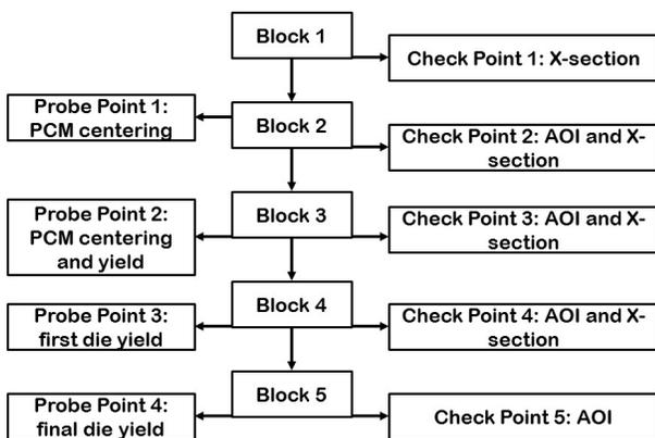
Figure 3. Simplified process flow with check points and their purposes
