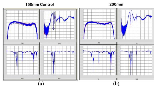
Figure 6. Pre and post stress RF performance comparison of one 200mm lot and one 150mm control lot
