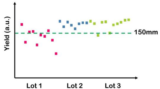
Figure 5. Wafer electrical die yield trend of the 200mm pathfinder lots (Square dots) vs the 150mm historical average (dotted line) for the same product.
