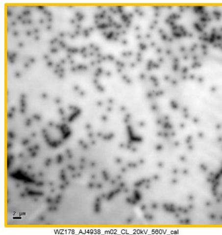
**Fig. 3. CL image from a 100 mm freestanding GaN substrate produced from a QST<sup>®</sup> seed. Average defect density measured in 4 spots was  $2 \text{E}7 \text{ cm}^{-2}$  with measurements ranging from  $1.61 \text{E}7$  to  $2.74 \text{E}7 \text{ cm}^{-2}$ .**
