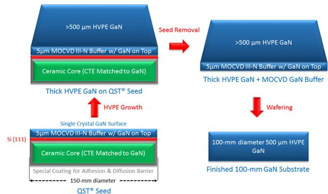
**Fig. 1. Schematic of the process beginning with a 150 mm QST<sup>®</sup> substrate as the seed (bottom left), followed by growth of thick HVPE GaN, then removal of the seed, then wafering to create a 100 mm diameter freestanding GaN substrate. The process can be applied to 200 mm QST<sup>®</sup> substrates to produce 150 mm diameter freestanding GaN substrates.**
