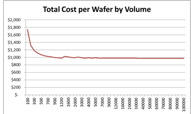
**Fig. 6. Cost of 150 mm freestanding GaN wafers by volume (per year) using the GaN-on-QST® seed approach.**
