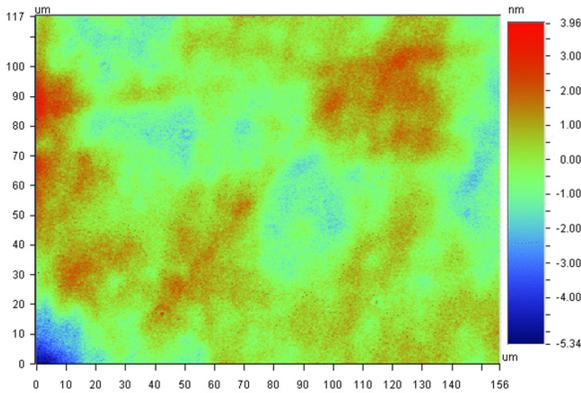
**Fig. 5. Wyko image of a the GaN surface after CMP, showing an  $R_q$  roughness of < 1 nm.**
