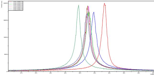
**Fig. 4. Omega scans across 90 mm of polished freestanding GaN (AJ4938) showing good potential within the inner 60 mm (average curvature > 35 meters corresponding to 9 μm of bow over 2” or 35 μm of bow over 4”) and lensing at the edge (with local curvature ~ 3 meters). The edge lensing stems from a polishing-induced mounting issue.**
