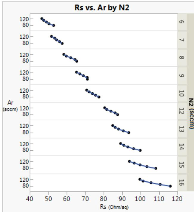
Figure 1. Gas ratio effect on  $R_s$ . General sheet resistance spread as a function of gas ratios across the entire process window. Note the distribution of points and general positive/negative trends.
