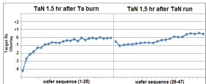
Figure 6. R<sub>s</sub> over time following a Ta “burn” sequence.
