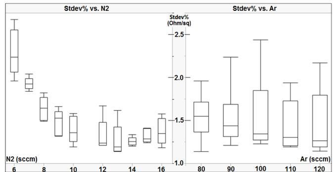
Figure 3. Uniformity distribution by gas flow. Variation in uniformity driven by  $N_2$ , not Ar.
