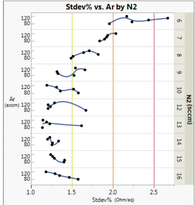
Figure 2. Gas ratio effect on uniformity.  $N_2$  is the main driver of uniformity. Time was held constant at 1 kW for all runs.
