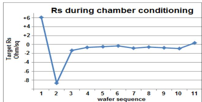
Figure 5. TaN run post chamber opening; no conditioning or target burn-in. (5 kW TaN process for 3 minutes in between wafers.)
