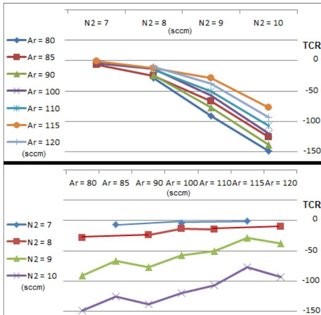
Figure 4. Gas flow effect on TCR. N<sub>2</sub> seen as primary contributor on resistor performance as TCR is an indicator of Ta: N<sub>2</sub> ratio, and therefore the particular phase of TaN.
