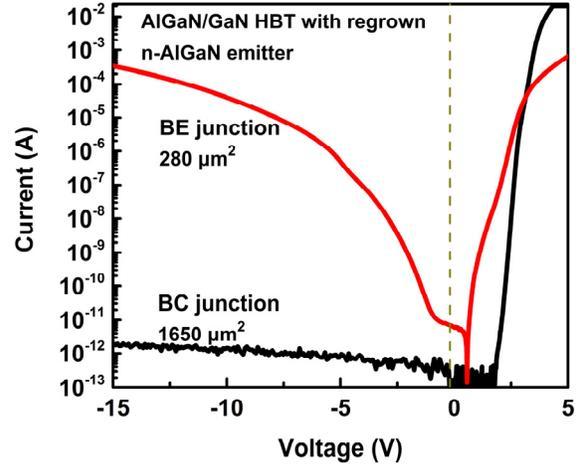
Fig. 4. The I-V characteristics of the base-collector junction and base-emitter junction of the AlGaIn/GaN HBT.
