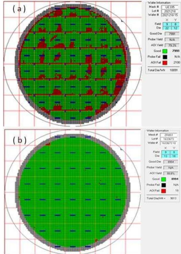
Fig. 3. (a) Gate integrity yield loss due to missing gates was typically seen at reticle field corners and (b) Optimized process gate integrity yield
