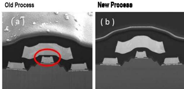
Fig. 6. Dielectric erosion improvement comparison. (a) Before process optimization and (b) Post process optimization
