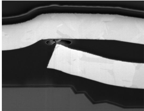
Fig. 5. Inter-level metal short due to photo resist and dielectric erosion during dry etch
