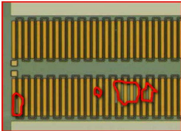
Fig. 2. pHEMT gate missing at reticle corner
