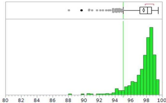
Fig. 7. Die-sort yield of a representative BiHEMT mask
