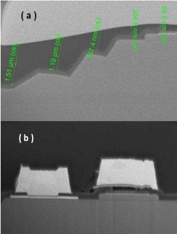
Fig. 4. (a) Very thin photo resist on top of HBT emitter due to high topology and (b) TaN metal deposited on top of HBT emitter, preventing the M1 from connecting the emitter
