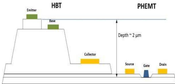
Fig. 1. BiHEMT schematic showing the severe device topology
