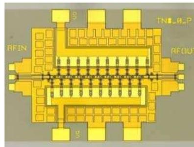
Fig. 4. Microphotograph of 1.0 THz TMIC amplifier.
