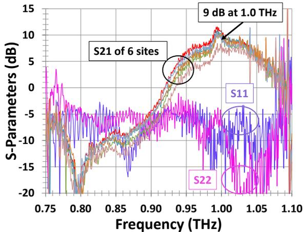
Fig. 5. On wafer measurement results showing 9 dB on-wafer gain at 1.0 THz.
