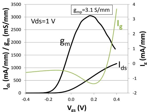
Fig. 2. DC transfer curves of a 2 finger 30  $\mu\text{m}$  device
