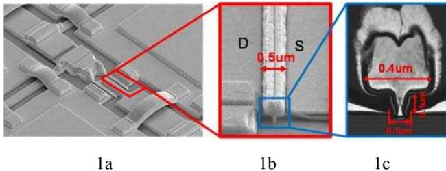
Fig. 1a. SEM image of TMIC; 1b. End view SEM of the transistor with 0.5  $\mu\text{m}$  source-drain distance; 1c. STEM image of the device cross-section.
