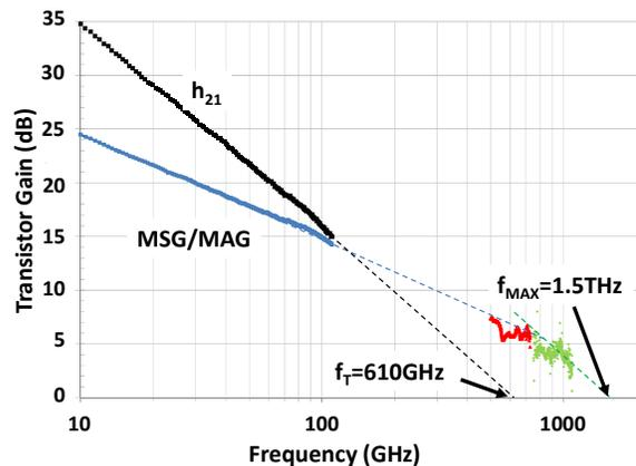
Fig. 3. Measured MAG/MSG and the associated  $h_{21}$  of a 2-finger 10  $\mu\text{m}$  device biased at  $V_{\text{d}}=1.2$  V and  $I_{\text{d}}=450$  mA/mm. The dashed lines represent data extrapolations with -20dB/decade and -10dB/decade slopes for the estimation of  $f_{\text{T}}$  and  $f_{\text{MAX}}$ .
